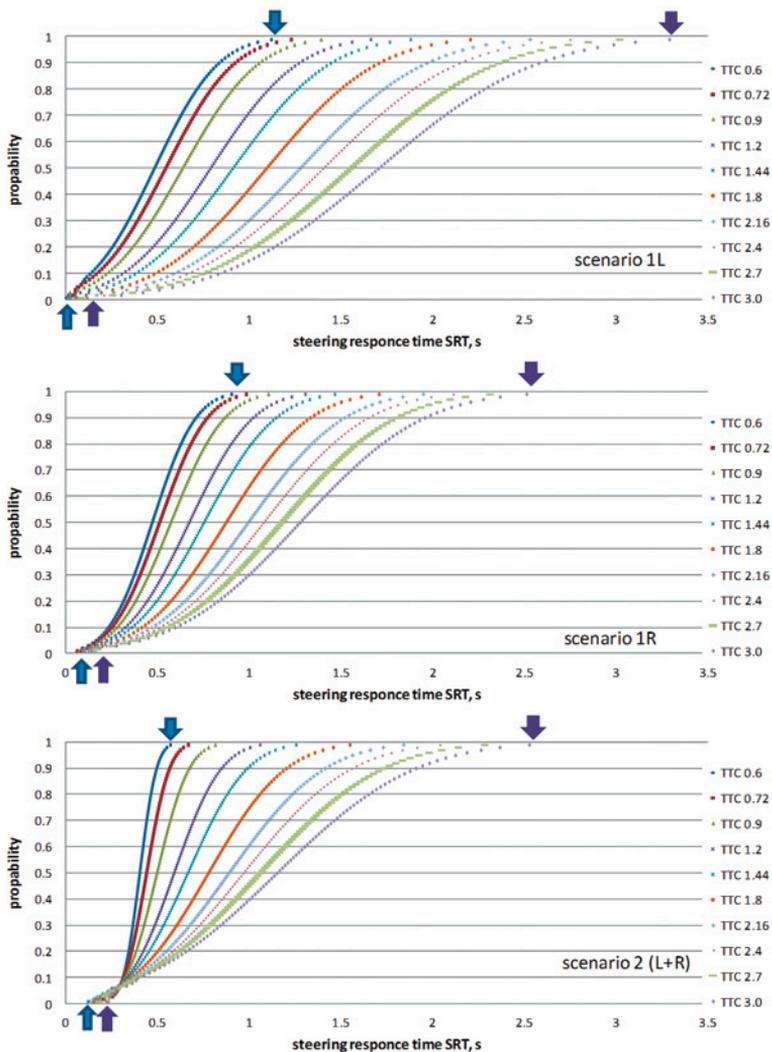
Fig. 8. Cumulative distribution functions for the steering response time (SRT)
