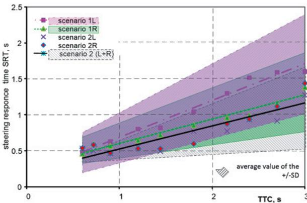
Fig. 7. Values of the steering response time (SRT)
