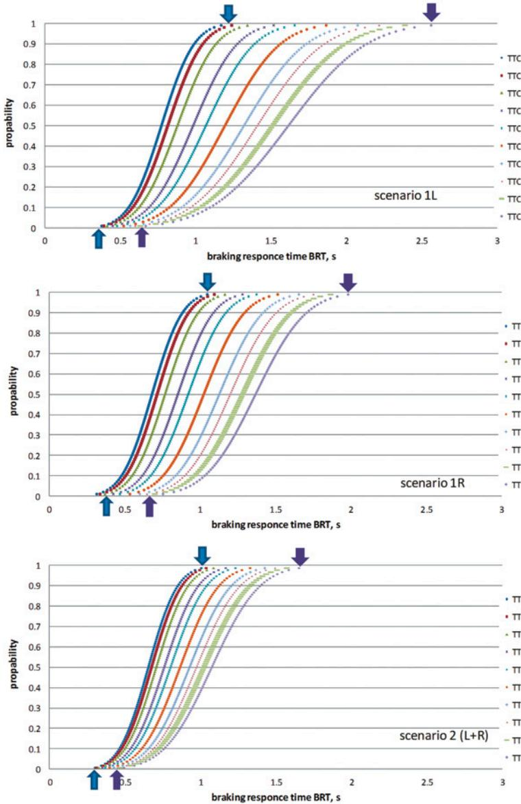
Fig. 6. Cumulative distribution functions for the braking response time (BRT)
