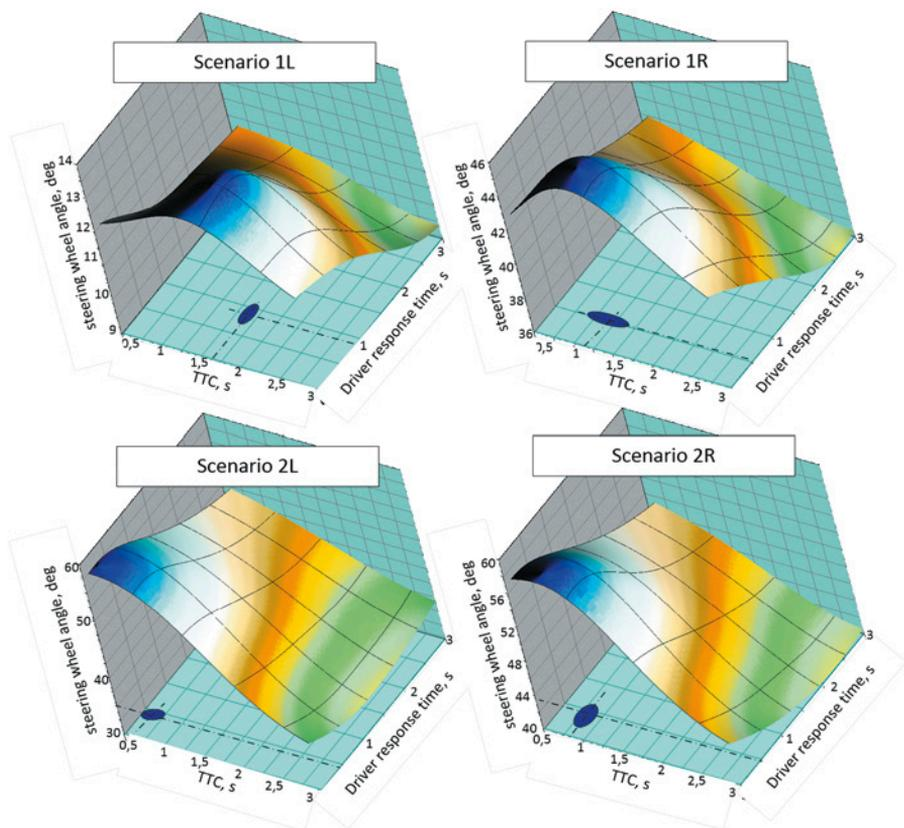
Fig. 14. Maximum steering wheel angle vs. TTC vs. driver steering response time (SRT)
