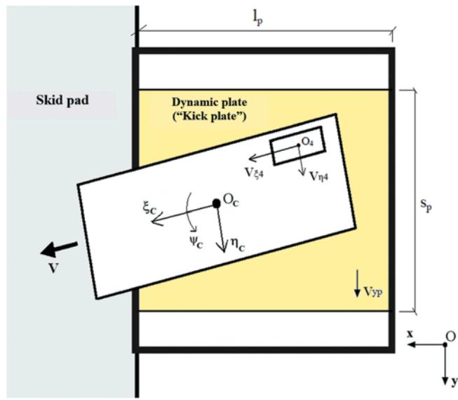
Fig. 1. Schematic diagram taken as a basis for the modification to the model and to the program simulating the vehicle motion on a DIC's test track provided with a skid pad and a dynamic plate ("kick plate") (see [2])
