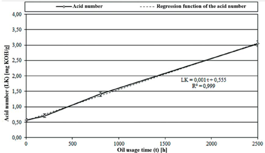
Fig. 3. Values of the acid number of hydraulic oil samples vs. oil usage time
