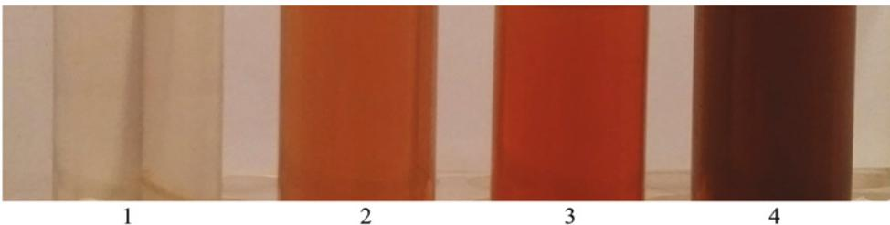
Fig. 1. Appearance of the hydraulic oil samples tested: 1 – fresh oil; 2 – oil having been used for 200 h; 3 – oil having been used for 800 h; 4 – oil having been used for 2 000 h
