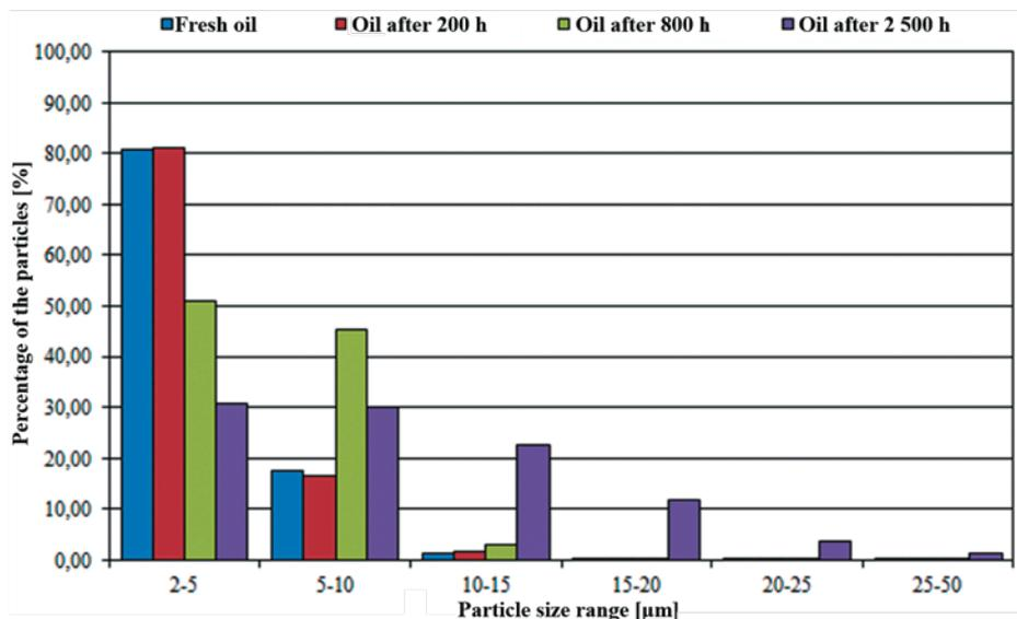
Fig. 5. Histogram of the percentage of contaminant particles of individual size ranges
