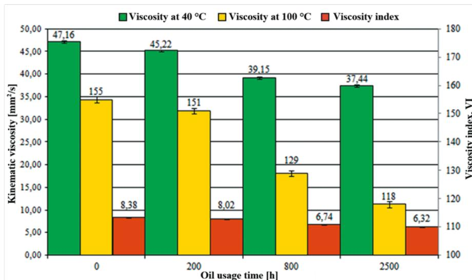
Fig. 2. Values of the rheological characteristics of hydraulic oil samples vs. oil usage time
