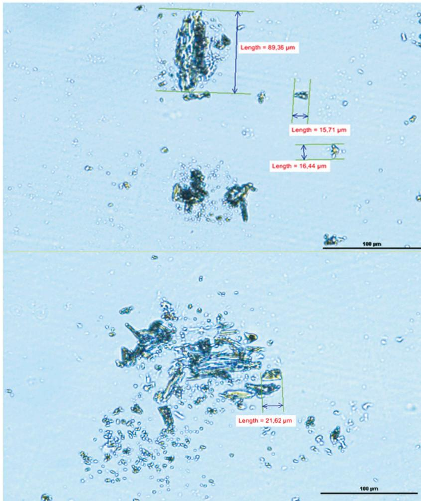
Fig. 6. View of contaminant particles in a hydraulic oil sample taken after 2 500 of use (magnification ratio: 20×10)
