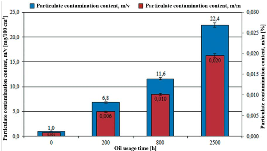
Fig. 4. Particulate contamination content of hydraulic oil samples vs. oil usage time
