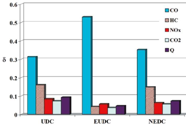
Fig. 6. The relative decrease rate in the specific distance emission of pollutants and operating fuel consumption due to additional supply of water to the operating medium
