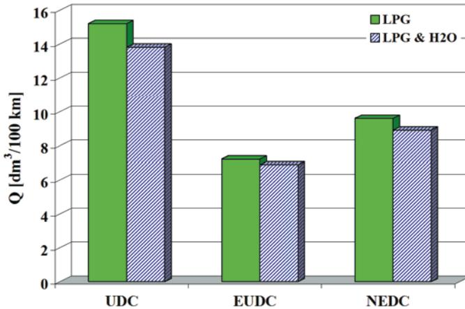
Fig. 5. Operating fuel consumption –  $Q$  during drive tests for two engine fuel systems
