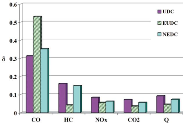
Fig. 7. The relative decrease rate in the specific distance emission of pollutants and operating fuel consumption due to additional supply of water to the operating medium
