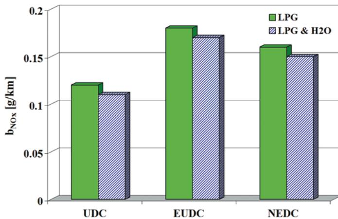
Fig. 3. Specific distance emission of nitrogen oxides -  $b_{NOx}$  during drive testing for two engine fuel systems
