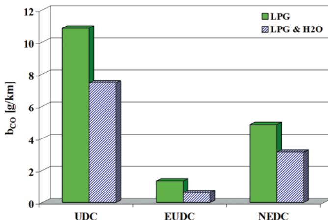
Fig. 1. Specific distance emission of carbon monoxide -  $b_{CO}$  during drive testing for two engine fuel systems
