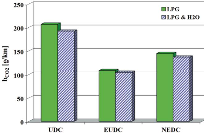
Fig. 4. Specific distance emission of nitrogen dioxide –  $b_{CO_2}$  during drive testing for two engine fuel systems
