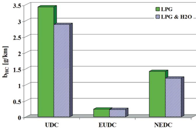
Fig. 2. Specific distance emission of hydrocarbons -  $b_{HC}$  during drive testing for two engine fuel systems
