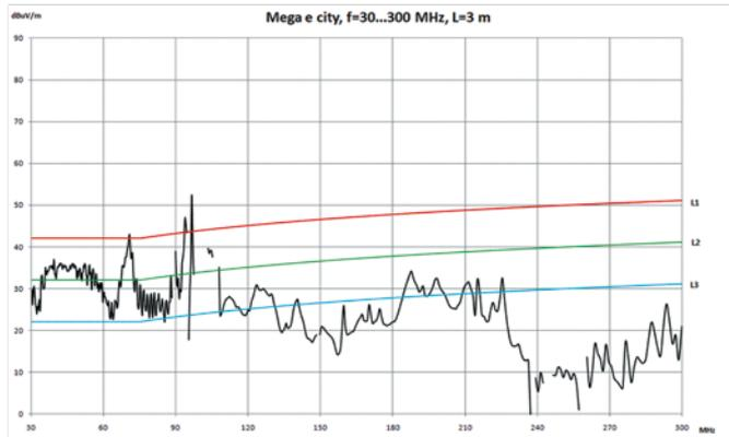
Fig. 9. Example curve representing the broadband emissions measured for the MEGA E CITY vehicle;
