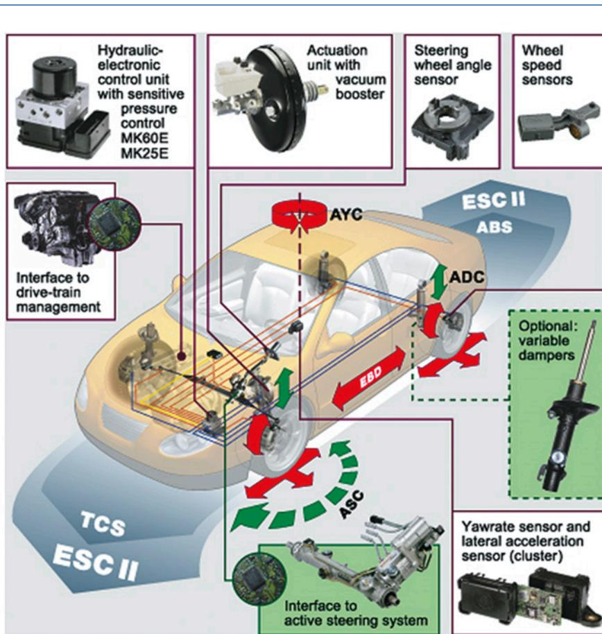
Fig. 3. Schematic diagram of the ESC II system [17]
