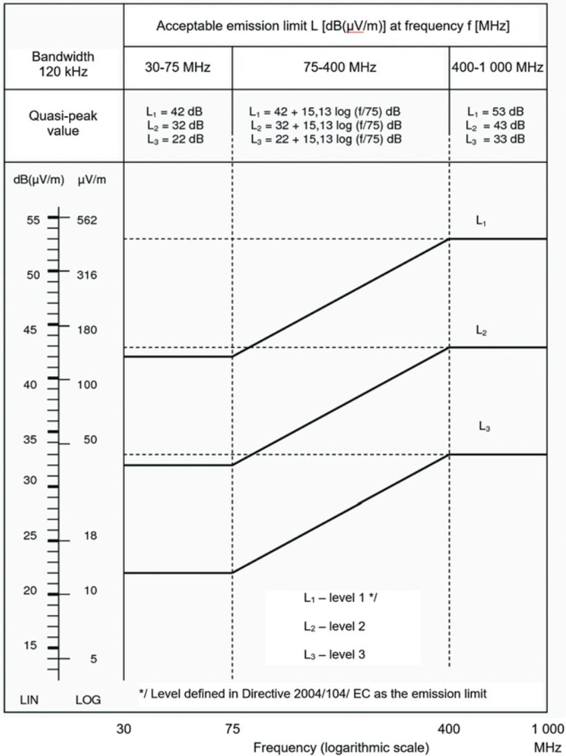
Fig. 2. Proposed reference levels of broadband electromagnetic emissions for vehicles
