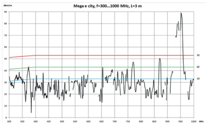
Fig. 10. Example curve representing the broadband emissions measured for the MEGA E CITY vehicle;
