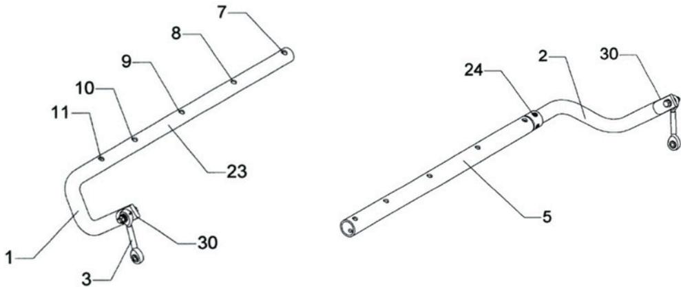
Fig. 6. Left: ground view of the smaller diameter stabilizer bar section. Left: ground view of the larger diameter stabilizer bar section. [5]
