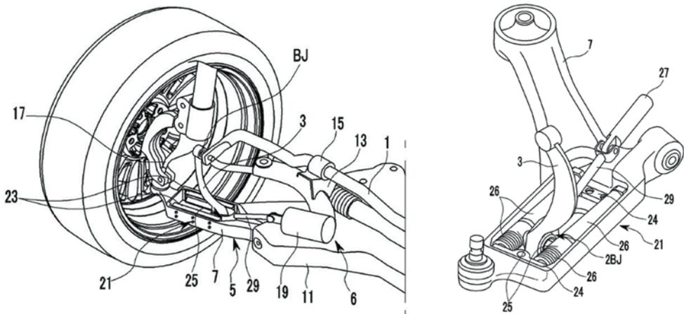
Fig. 11. Left: partial ground view on a vehicle suspension system with a rigidity shift mechanism installed. Right: ground view of the lower suspension arm with a modification to incorporate a sliding cavity [9]
