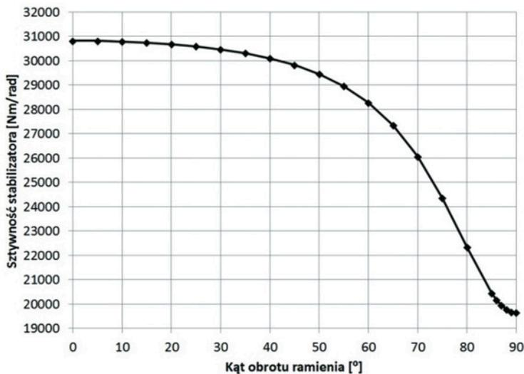
Fig. 10. Graph presenting the change of rigidity in a stabilizer of variable cross-section at the moment of being rotated to 90° from its vertical position to a horizontal position [own source]
