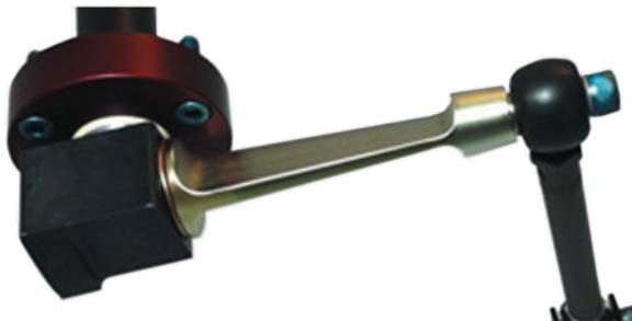
Fig. 9. Front stabilizer bar with adjustable arm [8]
