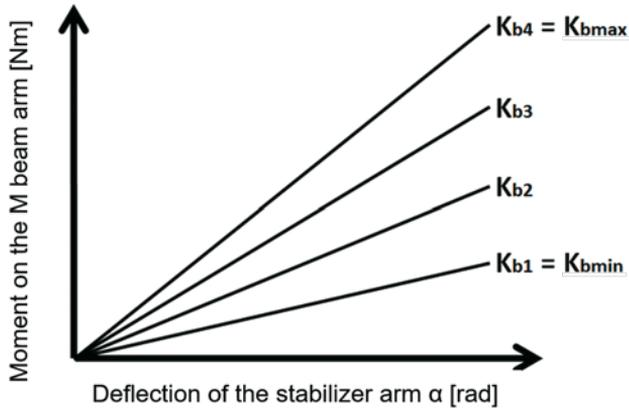
Fig. 2. The range of the active stabilizer rigidity alteration depending on its adjustment settings
