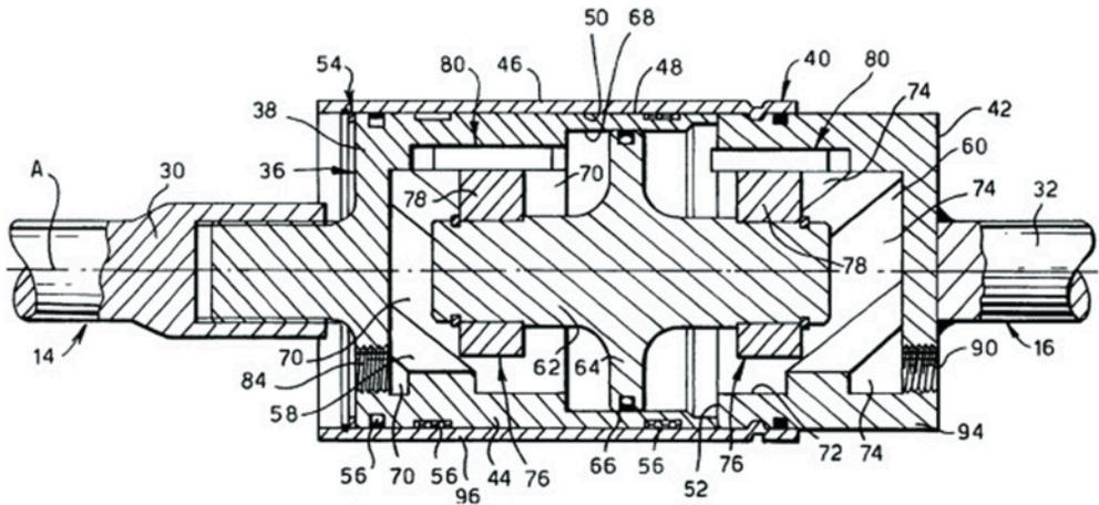
Fig. 5. Longitudinal section through a Delphi bar tensioning mechanism [4]
