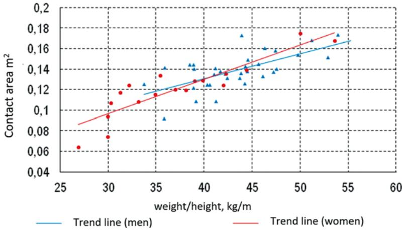
Fig. 8. Dependence between the contact surface area of the buttocks with the seat and the quotient of weight and height of persons participating in the research for a city car
