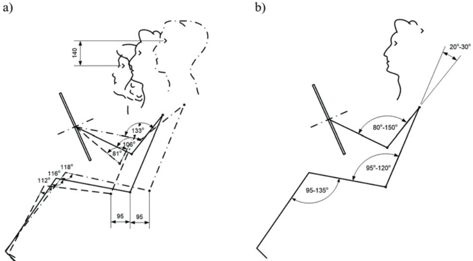
**Fig. 1. Comfort angles for sitting position in a car:**
