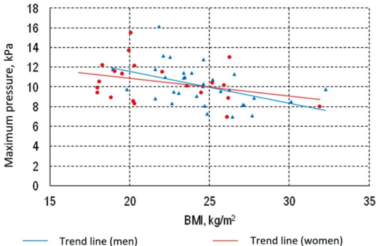
Fig. 11. Dependence between the maximum pressure imposed by the buttocks on the seat surface and the BMI of persons participating in the research for a mid-size car
