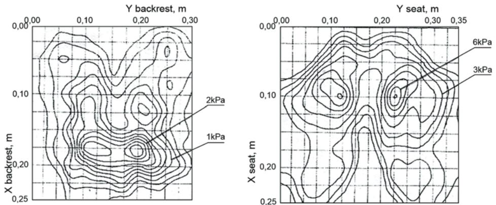
**Fig. 2. The example of pressure distribution on: a - backrest, b - seat bottom, of the comfortable seat**
