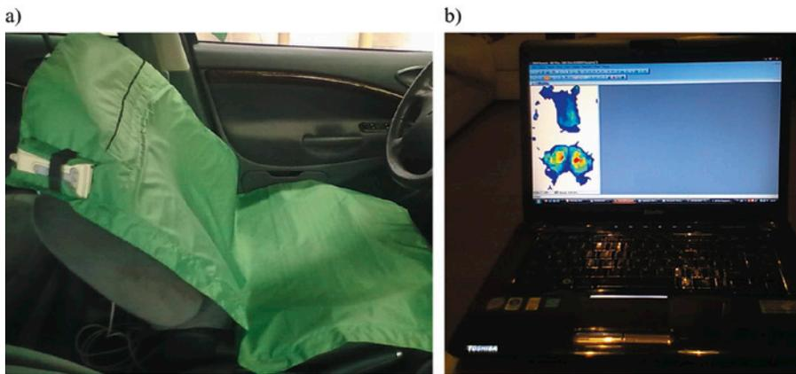
Fig. 3. Elements of measuring system: a) 5400N sensor (pressure sensing mat) placed on the seat with the Evolution Handle, b) PC with the software
