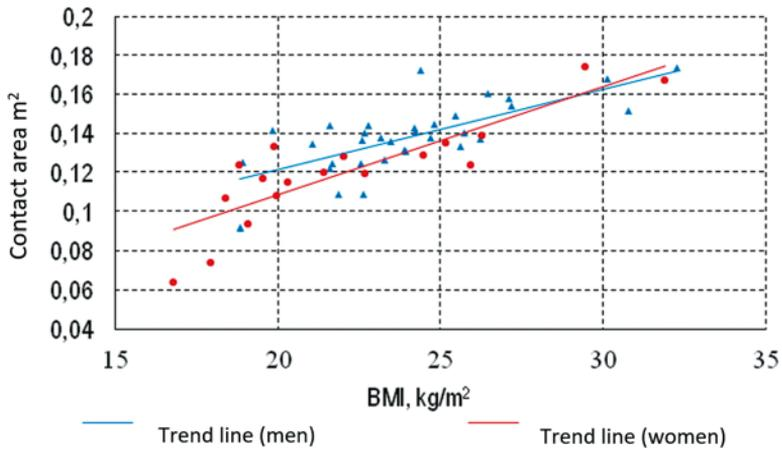
Fig. 6. Dependence between the size of the contact surface area of the buttocks with the seat and the BMI indicator of persons participating in the research for a city car
