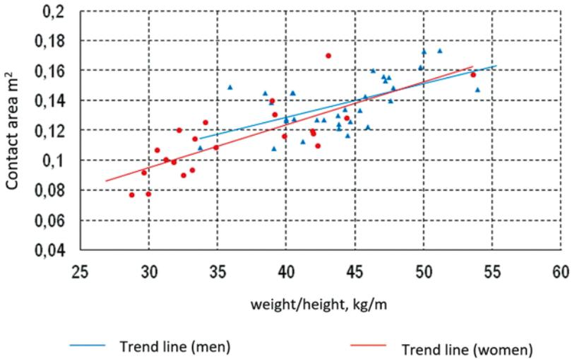
Fig. 9. Dependence between the contact surface area of the buttocks with the seat and the quotient of weight and height of persons participating in the research for a mid-size car
