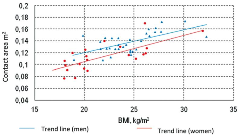
Fig. 7. Dependence between the size of the contact surface area of the buttocks with the seat and the BMI of persons participating in the research for a mid-size car
