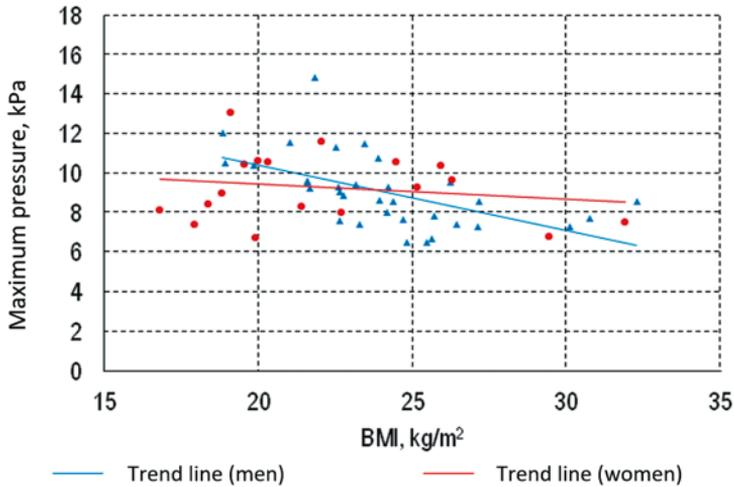
Fig. 10. Dependence between the maximum pressure imposed by the buttocks on the seat surface and the BMI indicator for persons participating in the research for a city car
