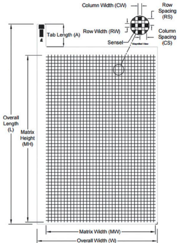
Fig. 4. Size of the pressure sensing mat model 5400N [12]
