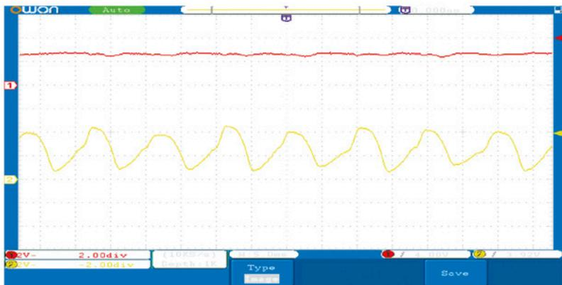
Fig. 8. Oscilloscope screen revealing Device I tendency to generate oscillations
