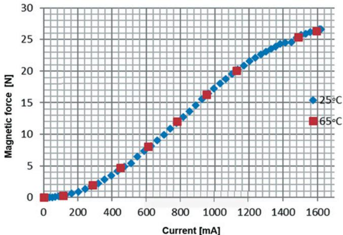
Fig. 13. Device I solenoid magnetic force measured for various temperatures and plotted vs. mean coil current
