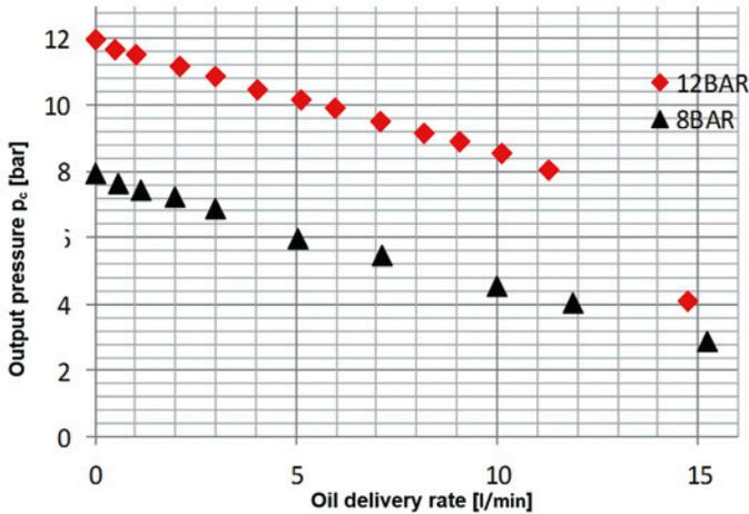
Fig. 16. Device I output pressure  $p_c$  vs. oil delivery rate for two initial output pressures,  $p_c=8$  bar and  $p_c=12$  bar. Supply pressure  $p_s = 15$  bar
