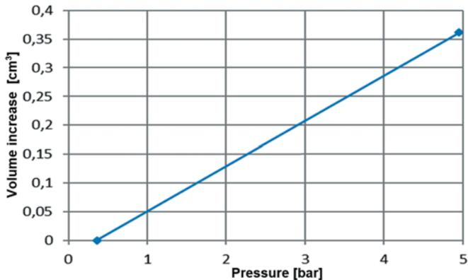
Fig. 7. Characteristic of the energy accumulator integrated into Device I
