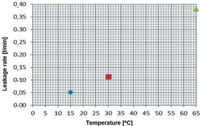
Fig. 15. Device I leakage rate vs. temperature
