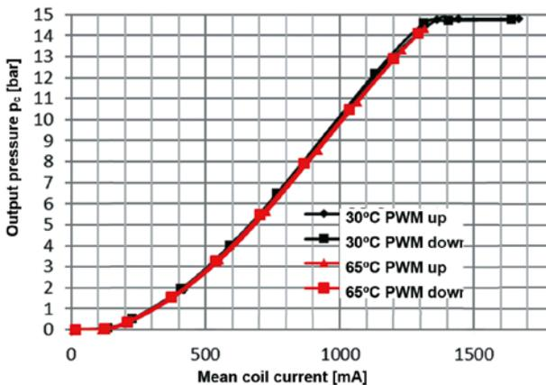
Fig. 12. Data from Fig. 10 plotted vs. mean coil current for various temperatures
