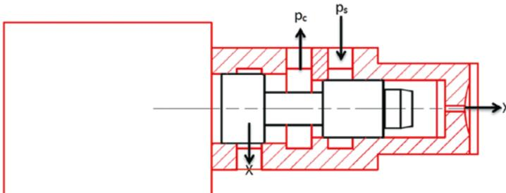
Fig. 4. Diagram showing the structure of solenoid valve, which is sufficient to perform the required functions
