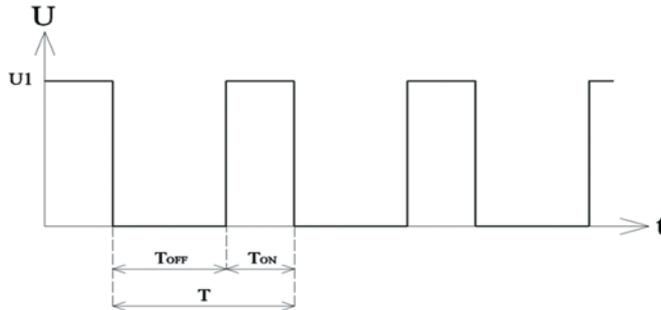
Fig.1. PWM control signal with period  $T$ , the period  $T_{on}$  when the signal is high (load is supplied), and the period  $T_{off}$  when the signal is low [12]
