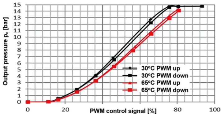
Fig. 10. Output pressure  $p_c$  produced by Device I vs. PWM control signal for various temperatures
