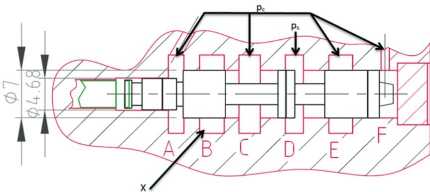
Fig. 6. Relative position of slider and the cylinder of the valve referred to as the Device I
