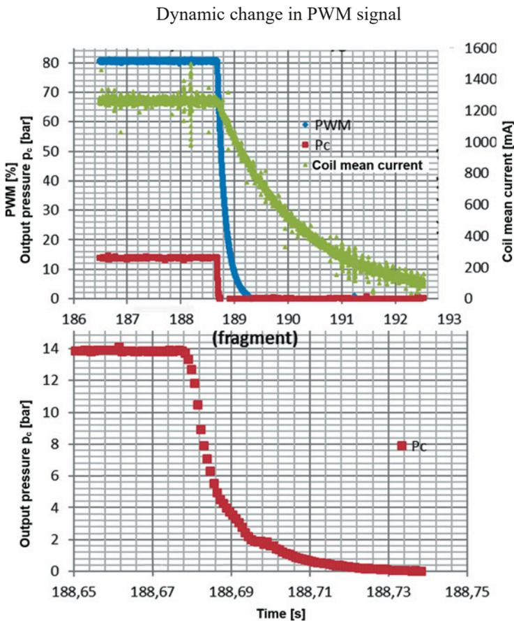
Fig. 14. Diagrams presenting dramatic changes of control signal in solenoid valve, referred to as Device I
