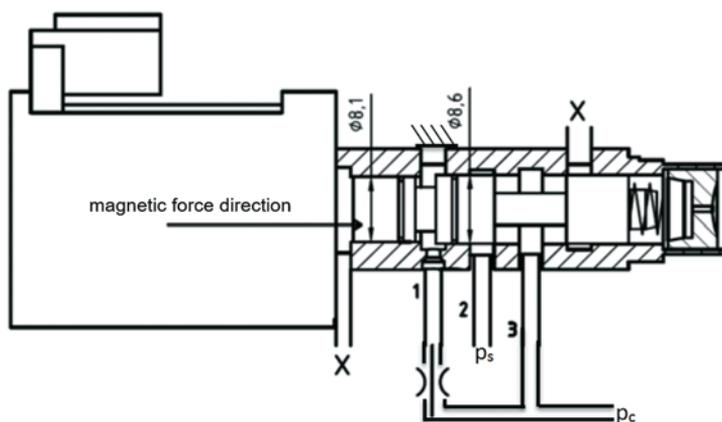
Fig.5. A diagram of the solenoid valve referred to as Device II
