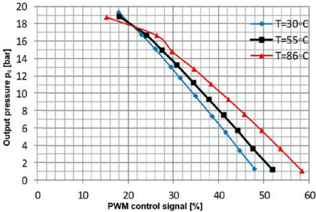
Fig. 11. Output pressure  $p_c$  produced by Device II vs. PWM control signal measured for various temperatures
