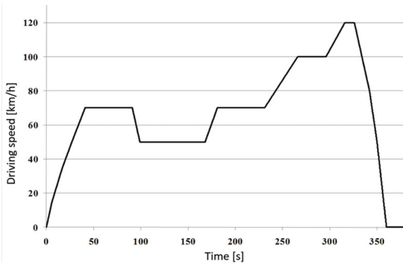
Fig. 19. Extra-urban operating conditions of a vehicle with electric drive
