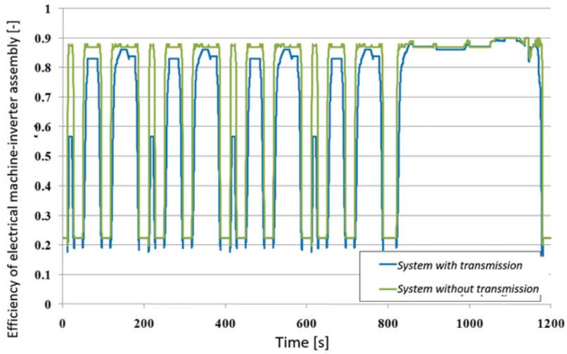
Fig. 15. The electric machine - inverter assembly efficiency
