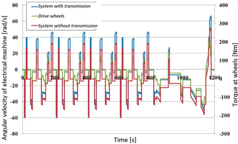
Fig. 11. The comparison of torque process for the drive wheels and the electric machine in an electric drive train system with a multi-speed transmission and without an additional transmission
