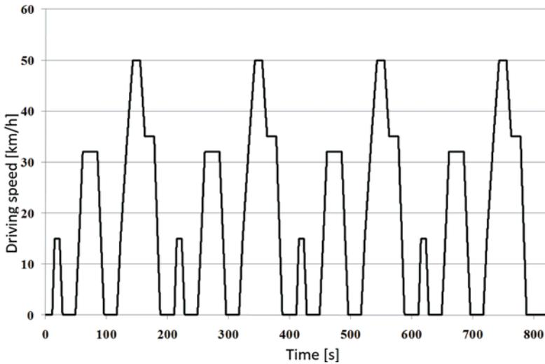
Fig. 18. Urban operating conditions of a vehicle with electric drive
