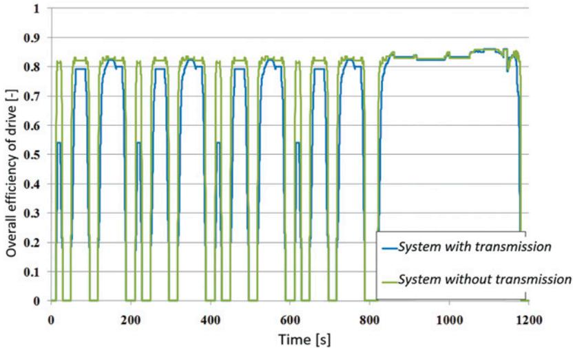
Fig. 17. The electric drive overall efficiency
