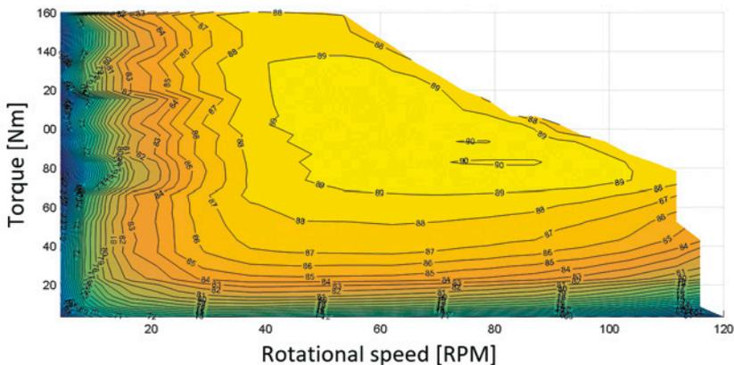
Fig. 4. Electric machine efficiency map relative to vehicle speed with the application of a single constant gear ratio
