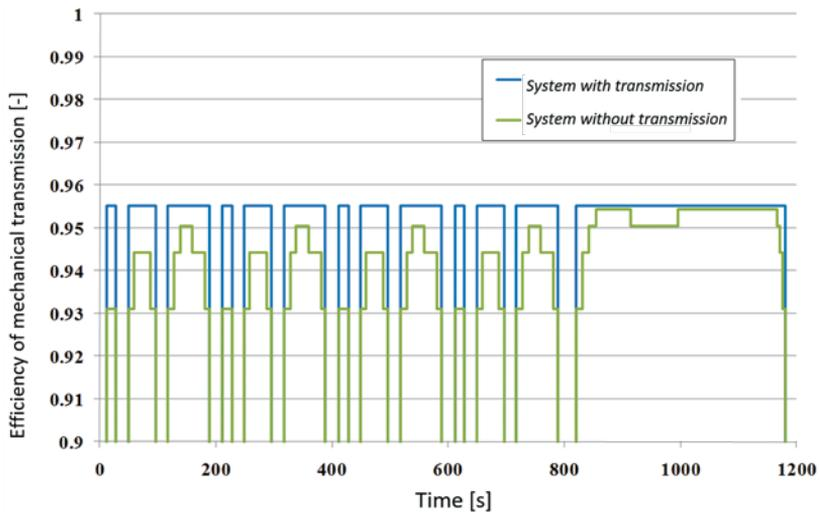
Fig. 16. The mechanical transmission overall efficiency
