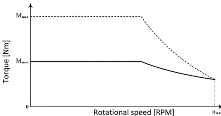
Fig. 2. The idea of electric machine overload
