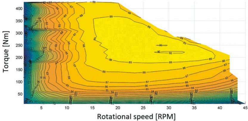
Fig. 5. Electric machine efficiency map relative to vehicle speed with the application of a constant gear ratio with limiting the maximum speed to approx. 50 km/h
