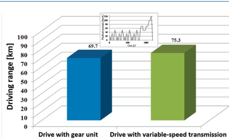
Fig. 14. The comparison of driving range for an electric drive train system vehicle with a multi-speed transmission and without an additional transmission
