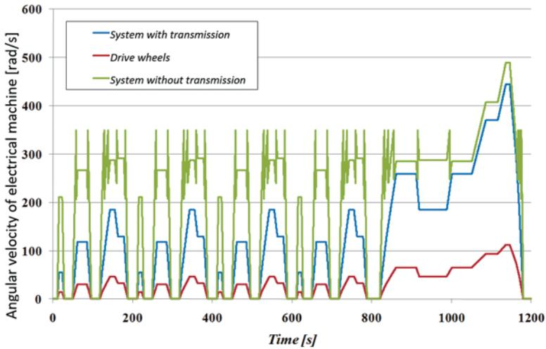
Fig. 10. The comparison of speed process for the drive wheels and the electric machine in an electric drive train system with a multi-speed transmission and without an additional transmission
