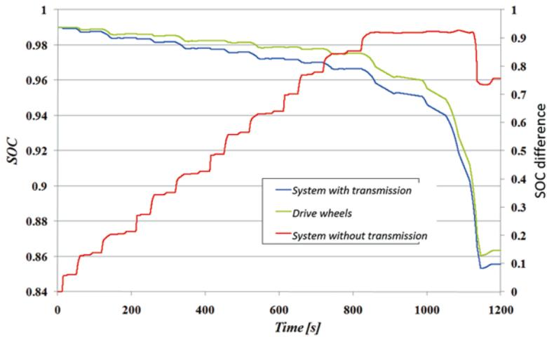
Fig. 13. The state of charge process (SOC) of an electrochemical battery featured in an electric drive train system with a multi-speed transmission and without an additional transmission
