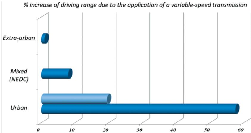
Fig. 22. The impact of the application of a multi-speed transmission on the driving range of an electric vehicle, depending on the operating conditions
