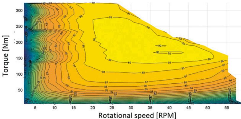
Fig. 6. Electric machine efficiency map relative to vehicle travel speed with the application of a gear ratio allowing high operation efficiency of the electric machine within a speed range of 40 km/h - 60 km/h
