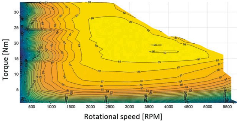
Fig. 3. Example efficiency map of a permanent magnet synchronous machine (PMSM)
