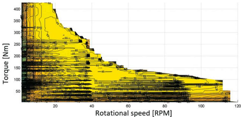
Fig. 7. Electric machine efficiency map relative to vehicle speed with the application of three gear ratios
