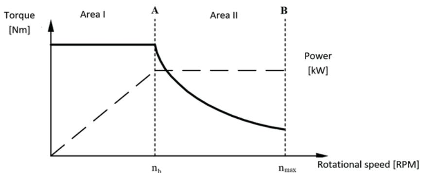
Fig. 1. The characteristics of the electrical machine controlled by PWM (Pulse Width Modulation) Method.
