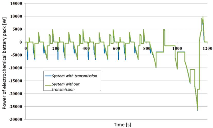
Fig. 12. The comparison of battery power process in an electric drive train system with a multi-speed transmission and without an additional transmission
