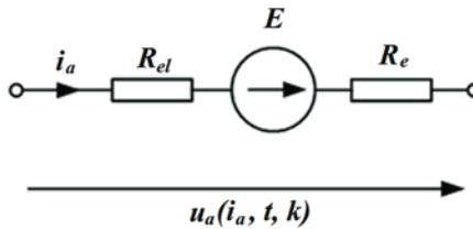
Fig. 8. Replacement diagram of electrochemical battery expressed by electromotive force  $E$  and non-linear resistance of electrodes  $R_c$  and electrolyte  $R_s$  dependent on the capacity of available battery (represented by charge level  $k$ );  $u(i_a, t, k)$  - voltage at battery terminals;  $t$  - time;  $k$  - battery charge coefficient;  $i_a$  - instantaneous battery current ([+] sign for discharge [-] for charging) [33,34]
