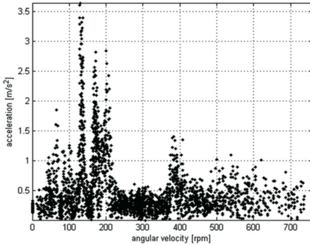
Fig. 8. Dependence of vibrations of the stand of the angular velocity of the left engine
