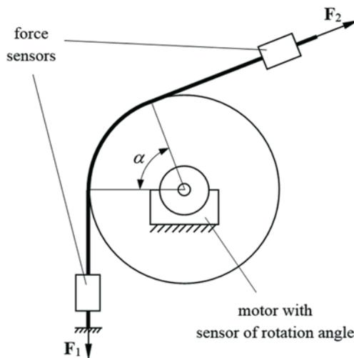
Fig. 4. Second configuration of the research stand which allows to measure the dynamic friction coefficient
