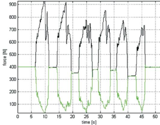
Fig. 11. Sample courses of the values of forces  $F_1$  and  $F_2$ , measured using the 2nd configuration of the stand:
