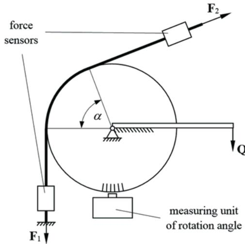
Fig. 2. First configuration of the research stand which allows to measure the static friction coefficient
