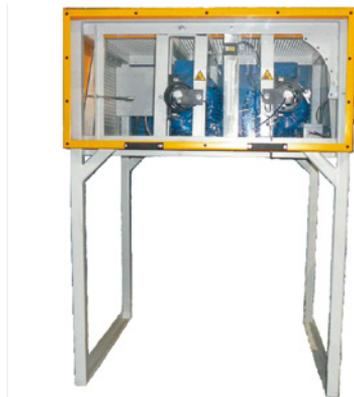
Fig. 1. Research stand for measuring friction in a belt transmission
