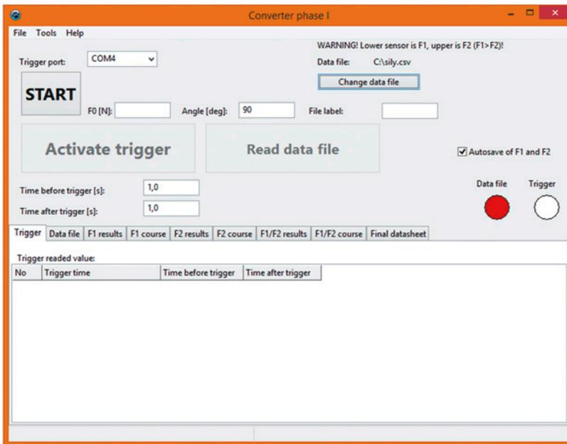
Fig. 3. Computer program for identification of forces  $F_1$  and  $F_2$  at moments of relative movement noticed between the belt and the pulley in the 1st configuration
