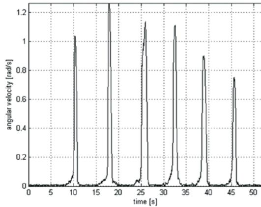
Fig. 12. Sample course of angular velocity measured using the 2nd configuration of the stand
