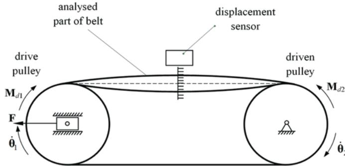
Fig. 6. Third configuration of the stand which allows to measure a complete belt transmission
