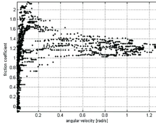
Fig. 13. Sample values of the friction coefficient as a function of the pulley angular velocity measured using the 2nd configuration of the stand
