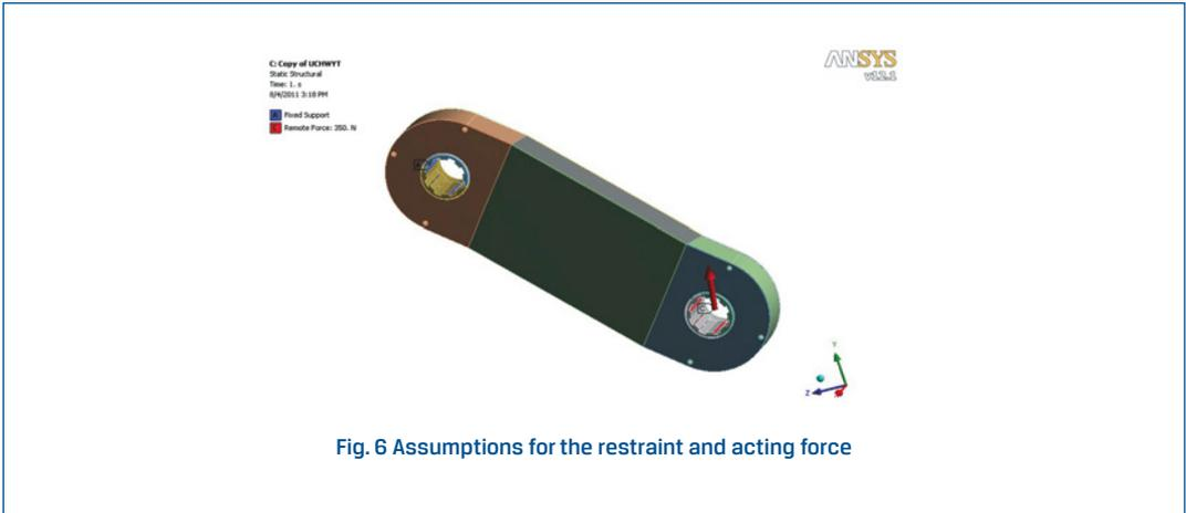
Figure 6 shows the restraint at the place marked with the letter A and the force acting on the suspension. This force was marked with the red arrow and the letter C.
