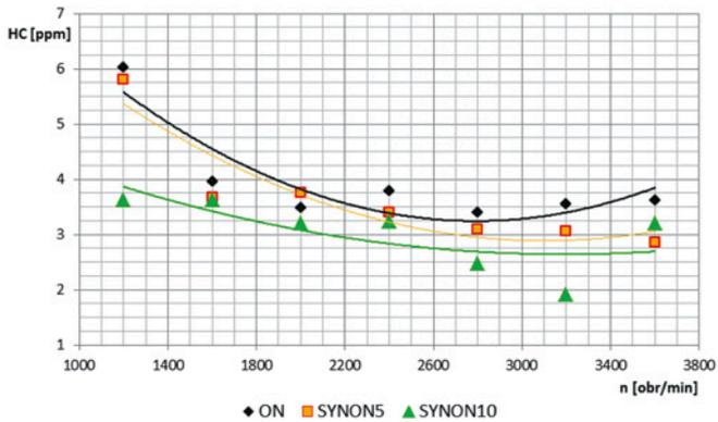
Fig. 7. Comparison of HC concentration in exhaust of AVL engine fuelled by mineral diesel fuel and mixtures of diesel fuel with synthetic hydrocarbons, working at full load
