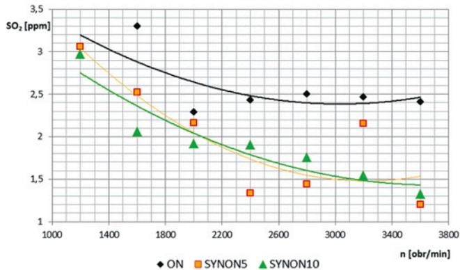
Fig. 9. Comparison of  $\text{SO}_2$  concentration in exhaust of AVL engines fuelled by diesel fuel and mixtures of diesel fuels with synthetic hydrocarbons, working at full load
