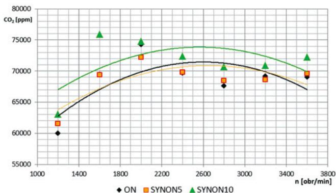
Fig. 5. Comparison of CO<sub>2</sub> concentration in exhaust from AVL engine which is fuelled by mineral diesel fuel and the mixtures of diesel fuel with synthetic hydrocarbons, working at full load
