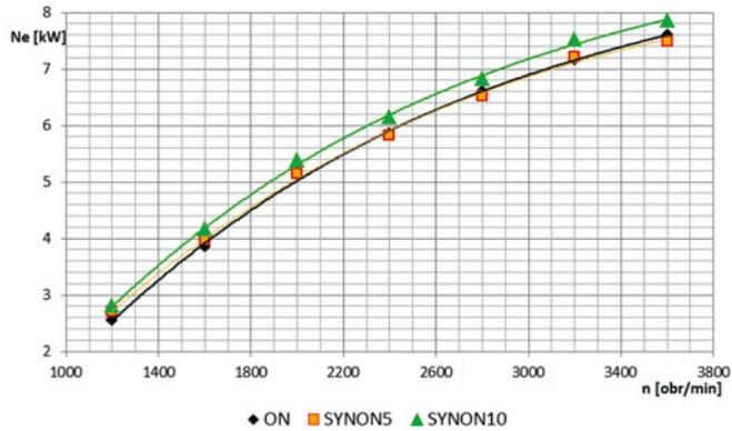
Figure 3. Comparison of effective power of AVL engine fuelled by mineral diesel fuel and mixtures of diesel fuel with synthetic diesel fuel, working at full load
