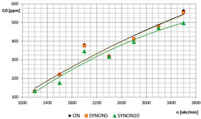
Fig. 6. Comparison of CO concentration in exhaust of AVL engine fuelled by mineral diesel fuel and mixtures of diesel fuel with synthetic hydrocarbons, working at full load
