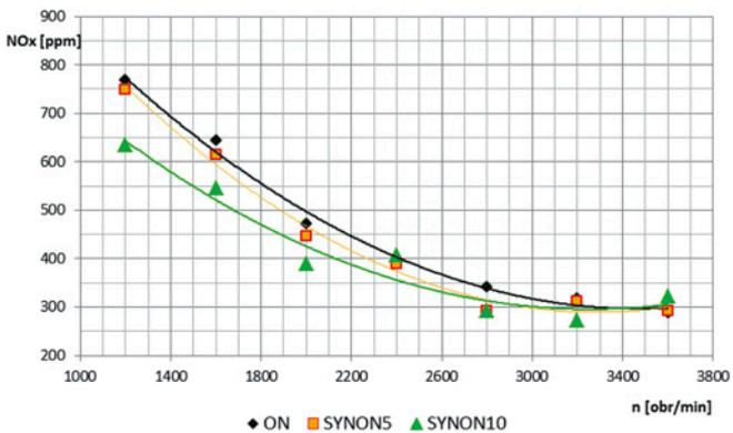
Fig. 8. Comparison of NO<sub>x</sub> concentration in exhaust of AVL engines fuelled by mineral diesel fuel and mixtures of diesel fuel with hydrocarbons, working at full load
