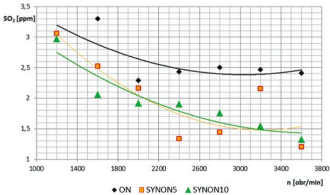
Fig. 9. Comparison of  $SO_2$  concentration in exhaust of AVL engines fuelled by diesel fuel and mixtures of diesel fuels with synthetic hydrocarbons, working at full load
