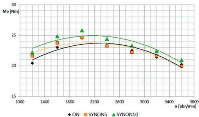
Figure 4. Comparison of torques of an AVL engine running on mineral diesel fuel and the mixture of diesel fuel and synthetic diesel fuel, working at full load
