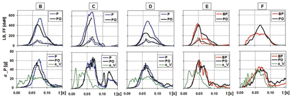
Fig. 16. Forces acting on the lap belt ( $LB$ ) and thighs ( $FF$ , fine lines), resultant pelvis acceleration ( $a_P$ ), and vehicle deceleration ( $a_V$ ) in tests B-F (in test C, variant PO, the  $LB$  force measuring system failed at the instant of about 0.07 s)
