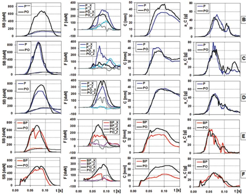
Fig. 11. Shoulder and thorax loads on the 10YO dummies in the vehicles used in tests B-F:
