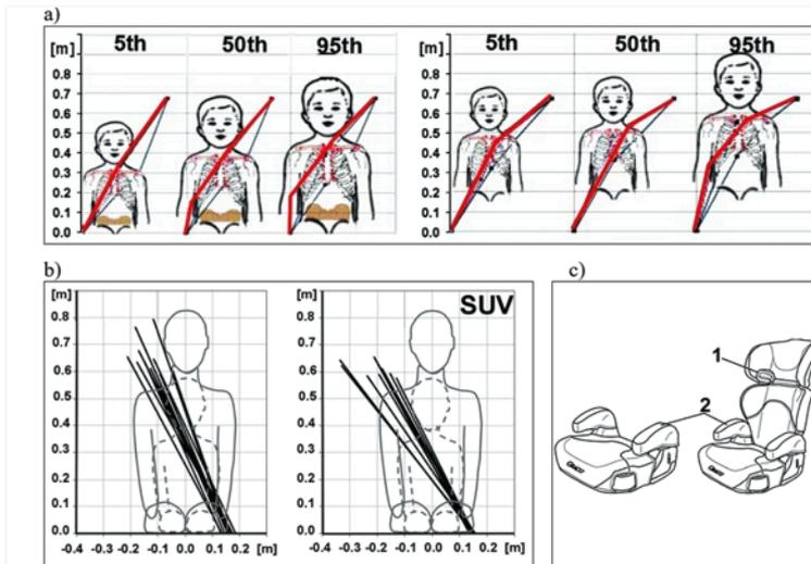
**Fig. 1. Positioning of the shoulder belt on child's torso: a) six-year-old child without a booster seat and sitting on a booster seat [2]; b) children aged 6 and 10 years in small passenger cars and in SUVs [3]; c) booster cushion (P) and high-back booster seat (PO) [8]; 1 – seatbelt guide; 2 – armrests**
