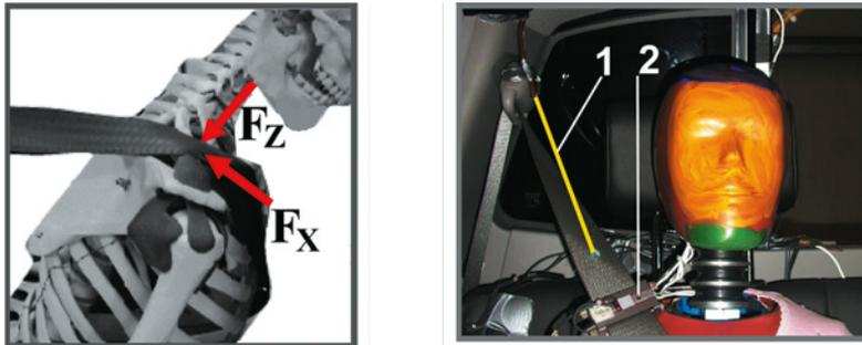
**Fig. 9. Position of the shoulder belt strap on dummy's shoulder and thorax and method of measuring the seatbelt strap displacement: 1 – cable of the seatbelt strap displacement transducer; 2 – SB force transducer on the shoulder belt strap [15, 28]**
