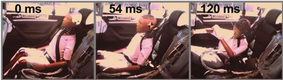
Fig. 13. Seatbelt position on the 10YO dummy in test G (based on [28])
