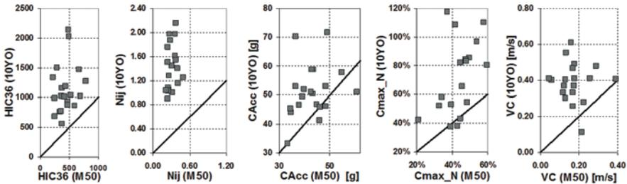
Fig. 2. Comparison of the injury indicator values determined for the driver (M50) and the child-passenger (10YO) occupying the rear vehicle seat; the straight lines represent the relation 1:1 [27]
