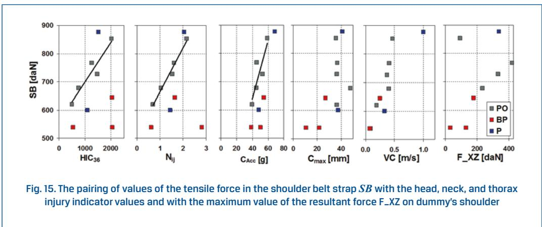
Fig. 15. The pairing of values of the tensile force in the shoulder belt strap  $SB$  with the head, neck, and thorax injury indicator values and with the maximum value of the resultant force  $F_{XZ}$  on dummy's shoulder
