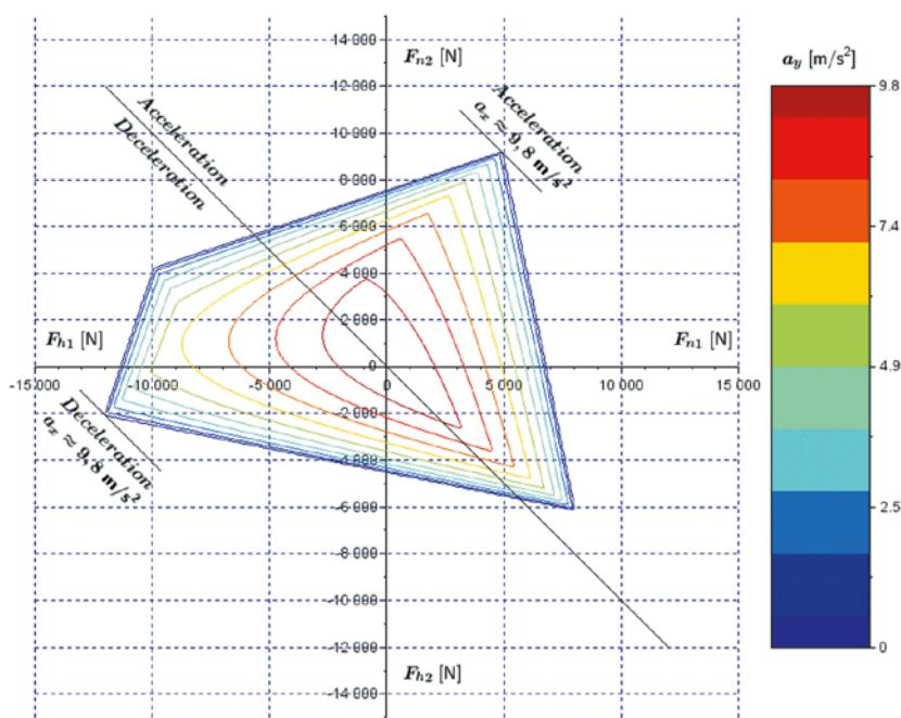
Fig. 3.2. The limit forces on wheels determined using the DSM method for  $h/l_{12} = 0.25$  ( $\mu_m = 1.0$ ;  $m_1/m_2 = 1.5$ )
