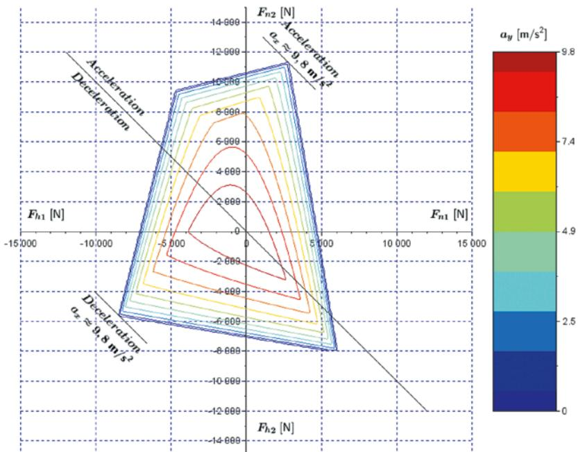
Fig. 4.2. The limit forces on wheels determined using the DSM method for the mass distribution to the axles of  $m_1/m_2 = 0.67$  ( $h/l_{12} = 0.2$ ,  $\mu_m = 1.0$ )
