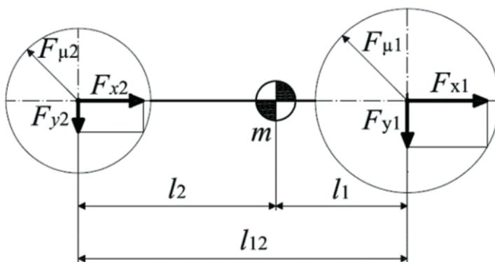
Fig. 2.1. The two-wheel vehicle model – top view
