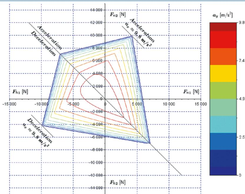
Fig. 4.1. The limit forces on wheels determined using the DSM method for the mass distribution to the axles of  $m_1/m_2 = 1.0$  ( $h/l_{12} = 0.2$ ,  $\mu_m = 1.0$ )
