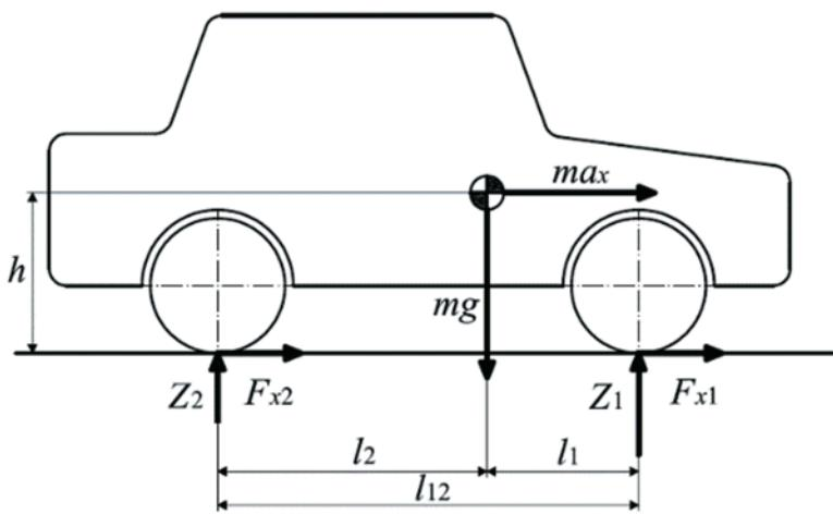
Fig. 2.2. The two-wheel vehicle model – side view
