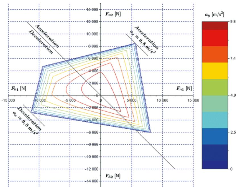
Fig. 2.4. The limit forces on wheels determined by the use of the DSM method for the reference vehicle
