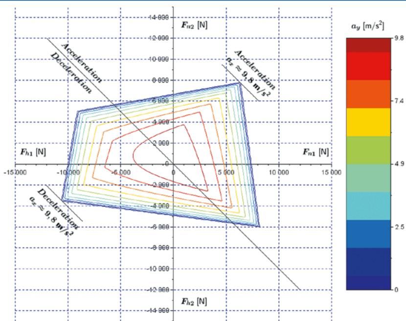
Fig. 3.1. The limit forces on wheels determined using the DSM method for  $h/l_{12} = 0.15$  ( $\mu_m = 1.0$ ;  $m_1/m_2 = 15$ )
