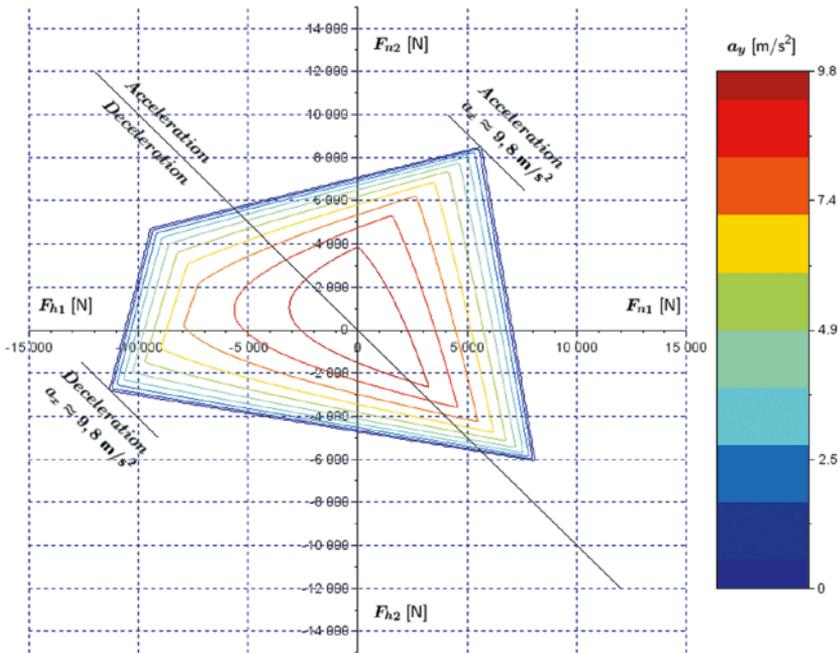
Fig. 2.4. The limit forces on wheels determined by the use of the DSM method for the reference vehicle ( $h/l_{12} = 0.2$ ;  $\mu m = 1.0$ ;  $m_1/m_2 = 1.5$ ) [1]
