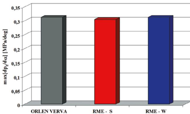
Fig. 9. Maximum values of the derivative of the indicated pressure with respect to the crank angle ( $\max[dp_g/d\alpha]$ ), averaged over the engine speed domain
