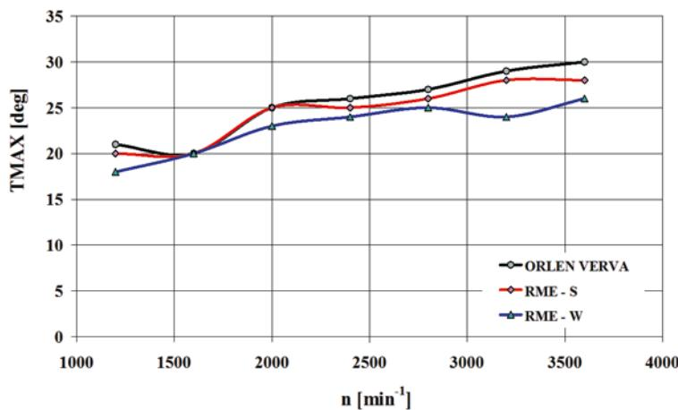
**Fig. 21.** Crank angle values corresponding to the maximum temperature of the working medium (TMAX) vs. engine speed (n)
