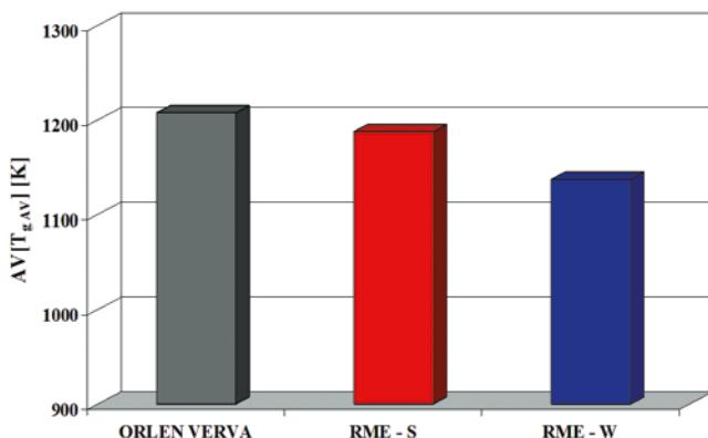
Fig. 19. Average values, taken for individual fuels over the engine speed domain, of the working medium temperature values averaged over the crank angle domain ( $AV[T_{gAV}]$ )
