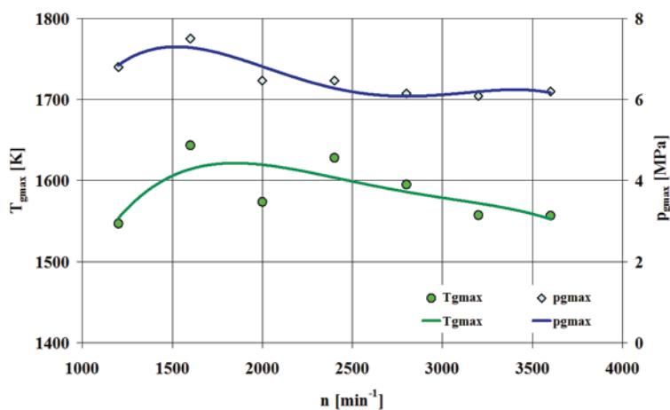
Fig. 14. Maximum temperature of the working medium ( $T_{\text{gmax}}$ ) and maximum indicated pressure ( $p_{\text{gmax}}$ ) vs. engine speed ( $n$ ) for the RME-S fuel
