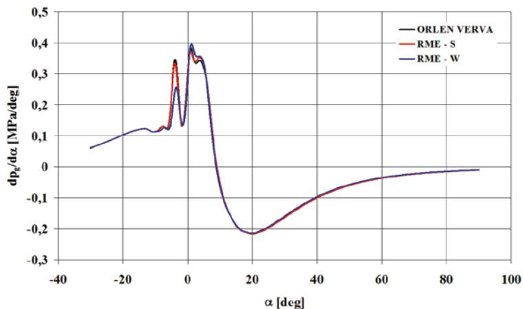
Fig. 4. Derivative of the indicated pressure with respect to the crank angle ( $\frac{dp_g}{d\alpha}$ ) for the maximum engine torque (at  $n = 1600 \text{ min}^{-1}$ )
