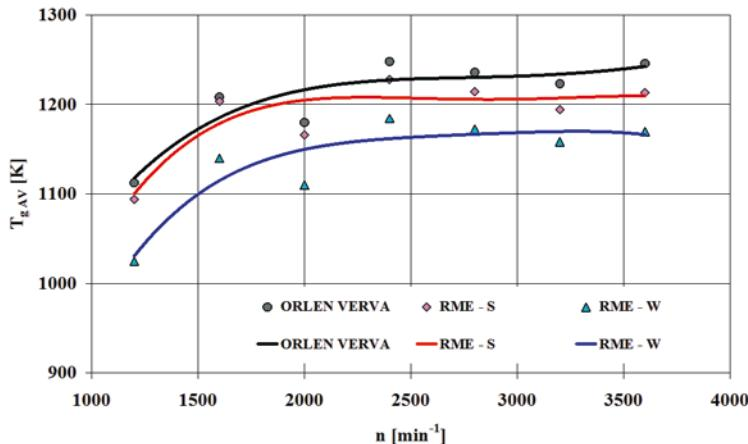
Fig. 18. Temperatures of the working medium averaged over the crank angle domain ( $T_{gAV}$ ) vs. engine speed (n)
