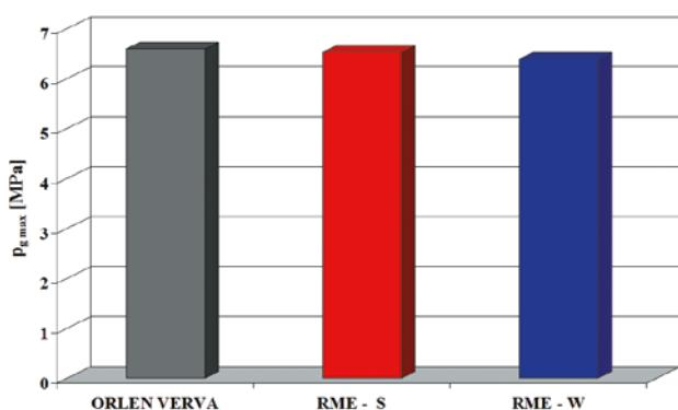
Fig. 8. Values of the maximum indicated pressure ( $p_{g\max}$ ), averaged over the engine speed domain
