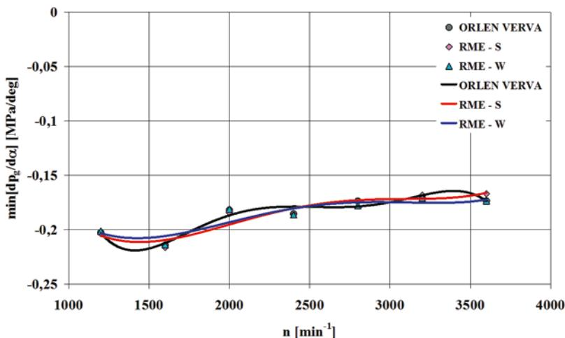
Fig. 7. Minimum values of the derivative of the indicated pressure with respect to the crank angle ( $\min[dp_g/d\alpha]$ ) vs. engine speed
