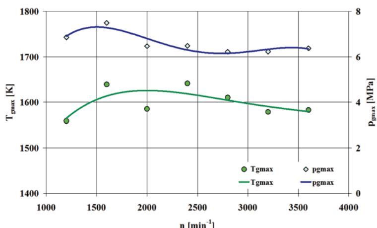
Fig. 13. Maximum temperature of the working medium ( $T_{g\max}$ ) and maximum indicated pressure ( $p_{g\max}$ ) vs. engine speed ( $n$ ) for the ORLEN VERVA fuel
