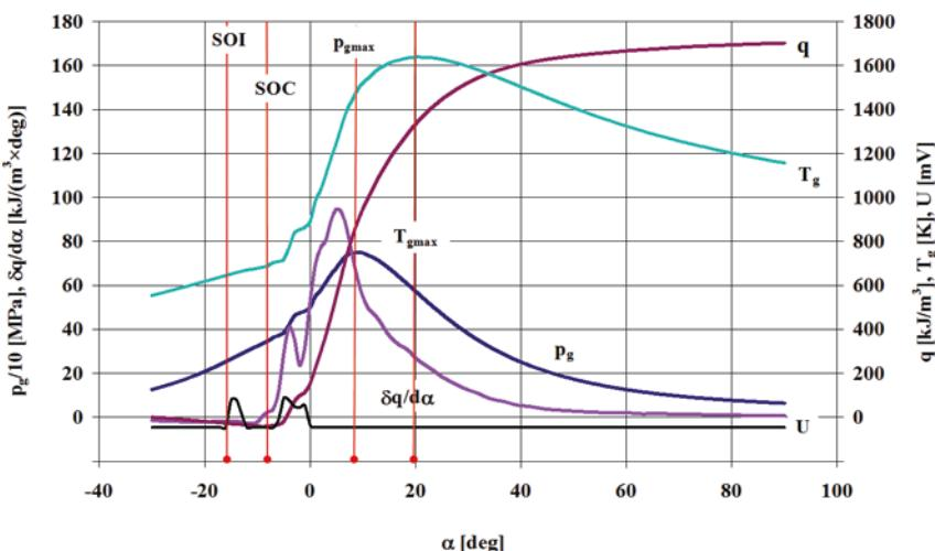
Fig. 11. Indicated pressure ( $p_g$ ), temperature of the working medium ( $T_g$ ), unit heat emission rate ( $\delta q/d\alpha$ ,  $\delta$  is the Pfaffian form), unit heat emission ( $q$ ), and injector opening control voltage ( $U$ ) for the maximum engine torque ( $n = 1600 \text{ min}^{-1}$ ) for the ORLEN VERVA fuel: SOI – fuel ignition start angle; SOC – combustion start angle;  $p_{g\max}$  – maximum indicated pressure;  $T_{g\max}$  – maximum temperature of the working medium
