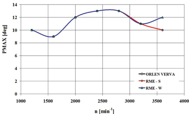
Fig. 20. Crank angle values corresponding to the maximum indicated pressure (P<sub>MAX</sub>) as functions of engine speed (n)
