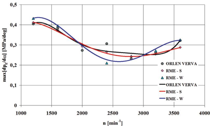
Fig. 6. Maximum values of the derivative of the indicated pressure with respect to the crank angle ( $\max[dp_g/d\alpha]$ ) vs. engine speed ( $n$ )
