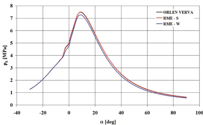
Fig. 3. Indicator diagram: indicated pressure ( $p_g$ ) for the maximum engine torque (at  $n = 1600 \text{ min}^{-1}$ )
