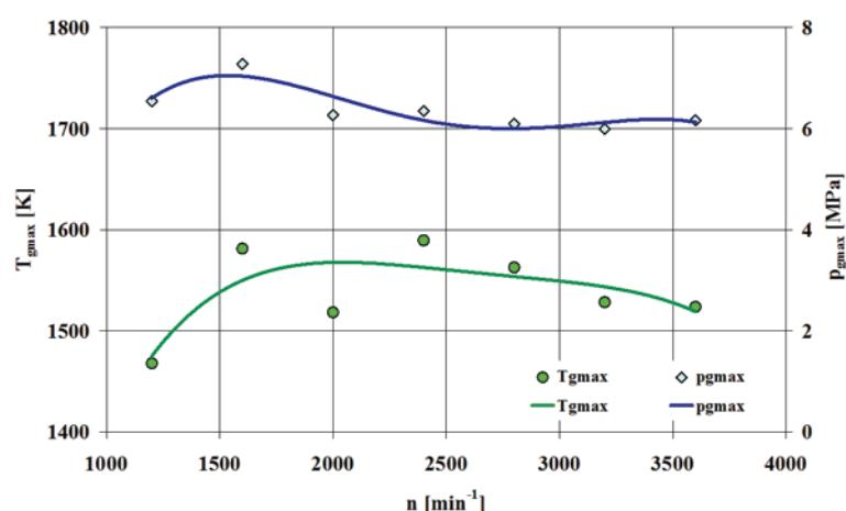
Fig. 15. Maximum temperature of the working medium ( $T_{\text{gmax}}$ ) and maximum indicated pressure ( $p_{\text{gmax}}$ ) vs. engine speed ( $n$ ) for the RME-W fuel
