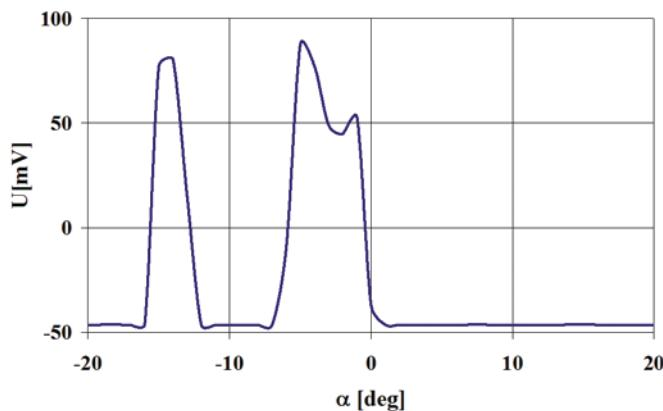
Fig. 1. Injector opening control voltage ( $U$ ) vs. the crank angle ( $\alpha$ ) measured from the top dead centre (TDC), at a point on the full-load power curve corresponding to an engine speed of  $1600 \text{ min}^{-1}$
