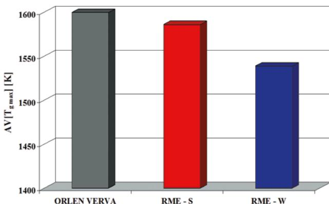
Fig. 17. Maximum temperature of the working medium, averaged over the engine speed domain (AV[T<sub>gmax</sub>])
