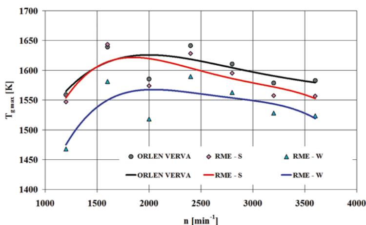
Fig. 12. Maximum temperatures of the working medium ( $T_{g\max}$ ) vs. engine speed ( $n$ )
