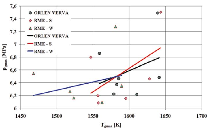
Fig. 16. Correlational interdependence between the maximum indicated pressure ( $P_{g\max}$ ) and the maximum temperature of the working medium ( $T_{g\max}$ )
