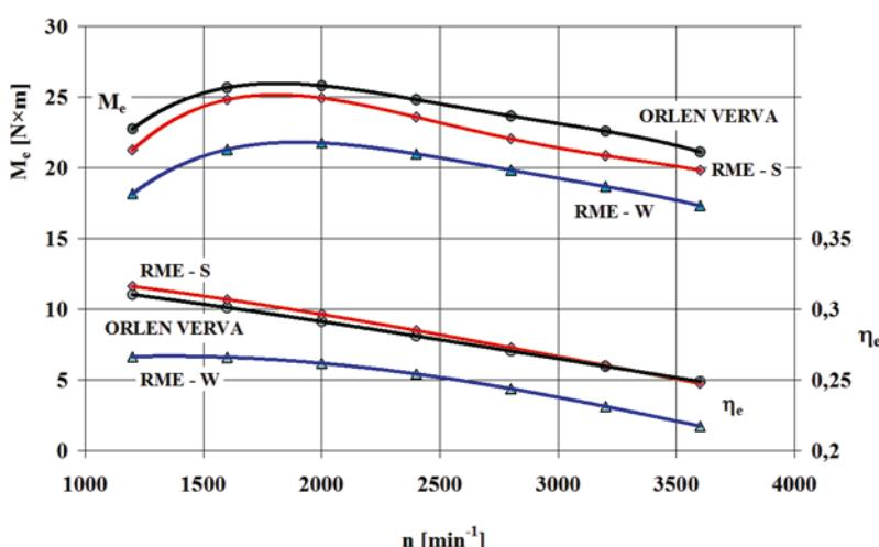
Fig. 2. Engine torque ( $M_e$ ) and effective efficiency ( $\eta_e$ ) vs. engine speed ( $n$ )
