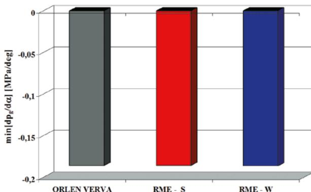
Fig. 10. Minimum values of the derivative of the indicated pressure with respect to the crank angle ( $\min[dp_g/d\alpha]$ ), averaged over the engine speed domain
