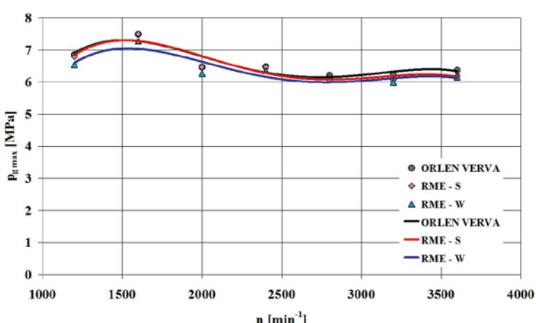
Fig. 5. Maximum indicated pressure ( $p_{g\max}$ ) vs. engine speed ( $n$ )
