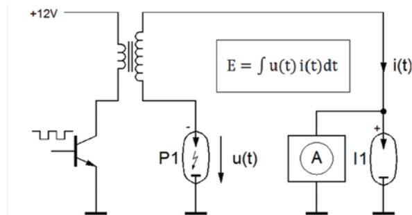
Fig. 5. Schematic diagram of measuring the spark discharge energy of a spark plug featuring a negative polarity electrode
