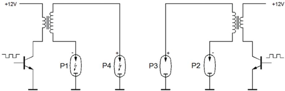
Fig. 3. Distributorless ignition system of a four-cylinder engine featuring a double-ended coil
