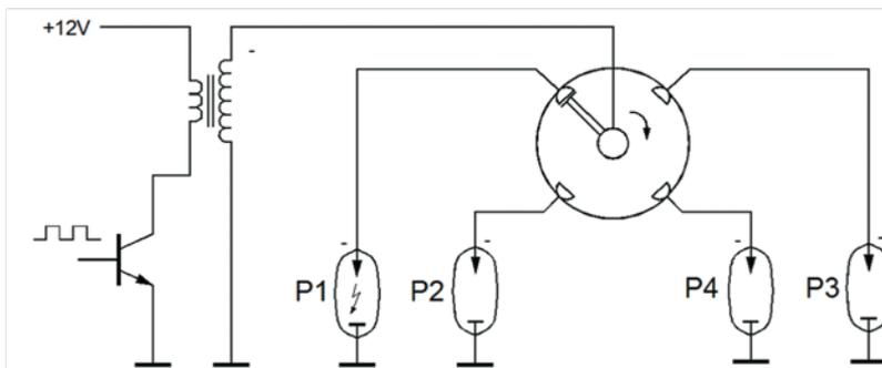
Fig. 1. Ignition system with a distributor mechanism
