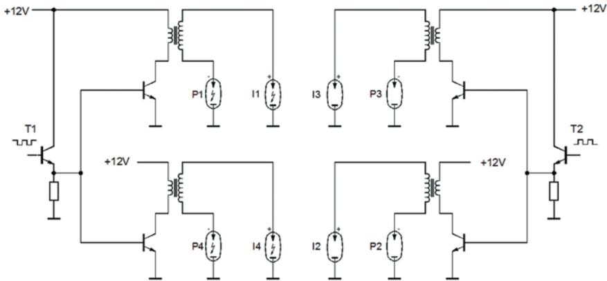
Fig. 4. The solution to the issue of ensuring uniform polarity of central spark plug electrodes in a circuit featuring double-ended coils
