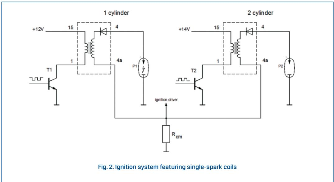
Fig. 2. Ignition system featuring single-spark coils
