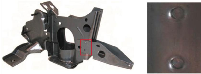
Fig. 20. Brake pedal supporting structure
