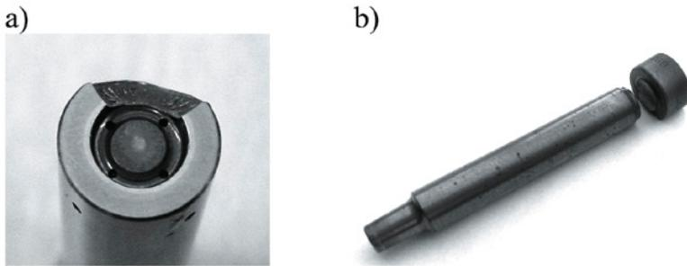
Fig. 8. Tools for the forming of a clinched joint, withdrawn from service: a) – die; b) – punch
