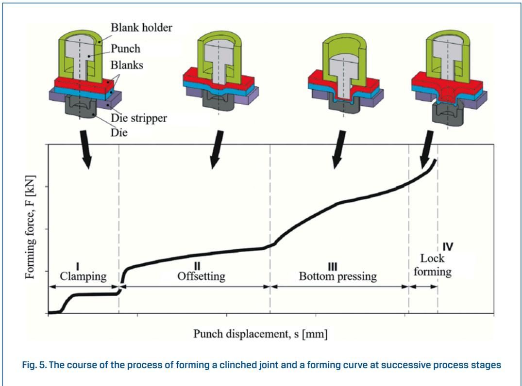
Fig. 5. The course of the process of forming a clinched joint and a forming curve at successive process stages
