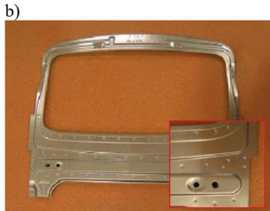
Fig. 21. Clinched joints: a) – in a clutch shell; b) – in a sunroof component
