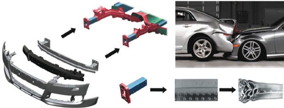
Fig. 26. Modelling and crash-testing of the vehicle body structures with clinched joints
