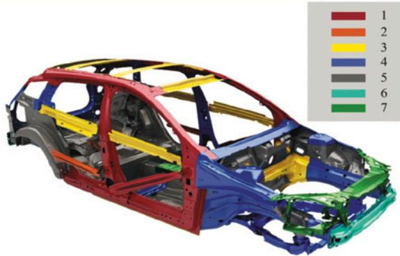
Fig. 1. An example of using different construction materials for motor vehicle body components: 1 – magnesium alloys; 2 – aluminium alloys; 3 – low-carbon deep-drawing steels; 4 – higher-strength steels HSS; 5 – high-strength steels; 6 – very high-strength steels; 7 – ultrahigh-strength steels
