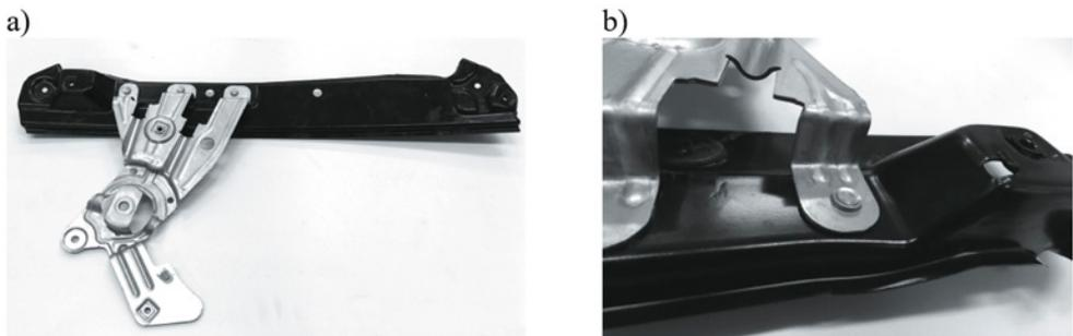
Fig. 15. Fragments of a door window lifting linkage: a) – supporting structure; b) – clinched joint, viewed facing the side formed by the die
