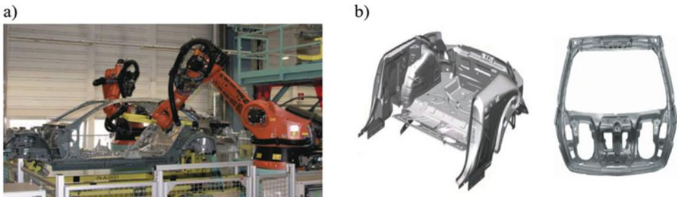
Fig. 10. Example of the assembly of Audi TT Coupé body components: a) – assembly workstation; b) – body components assembled with the use of the CL technology
