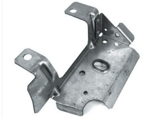
Fig. 18. A fastening portion of a bracket structure installed in the engine compartment
