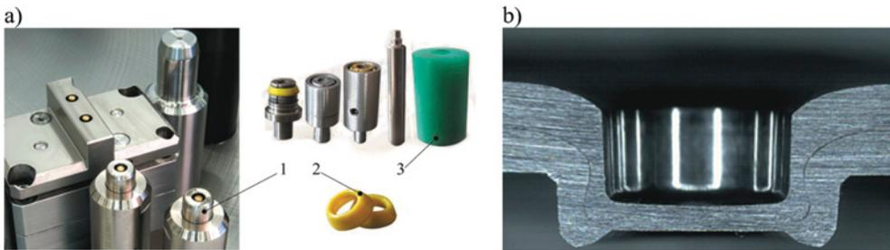
Fig. 6. Example joint-forming tools (a) and the cross-section of a joint formed with the use of a round solid die (b): 1 – punch in a blank-holding sleeve with a spring; 2 – elastomer ring of the die with movable segments; 3 – blank-holding elastomer sleeve
