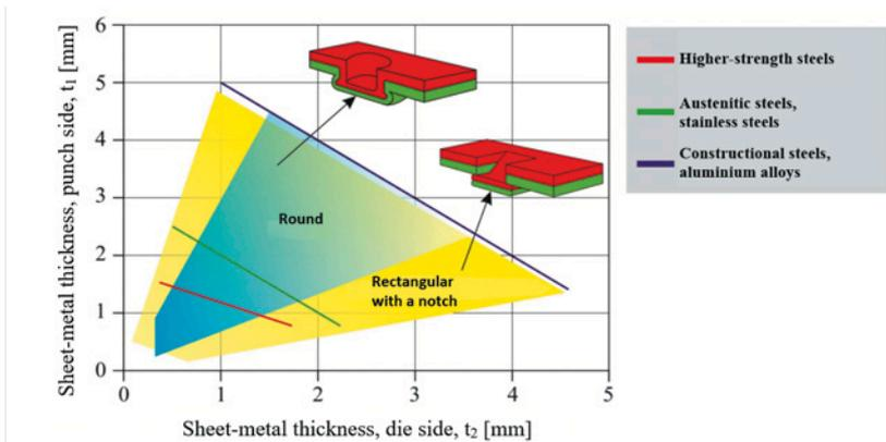
Fig. 7. Strength of the joints formed with the use of various tools
