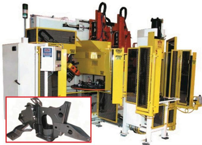
Fig. 12. Specialized machine for fixing a pedal bracket in a passenger car (a solution adopted by BTM Corporation)
