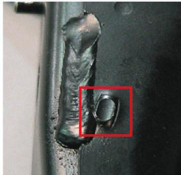
Fig. 14. Rectangular clinched joint used for the preliminary fixing of parts before their final bonding
