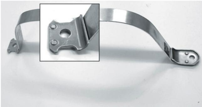
Fig. 17. Fuel tank mounting strap
