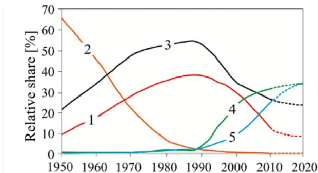
Fig. 4. Share of individual joining techniques used for the production of motor vehicle bodies: 1 - MIG/MAG welding; 2 - gas brazing; 3 - resistance welding; 4 - clinching; 5 - laser-beam welding (based on: IWU Fraunhofer Institute)
