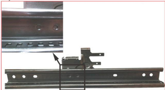
Fig. 19. Implementation of clinched joints in the construction of a vehicle seat: a) – seat frame; b) – seat sliding runner subassembly
