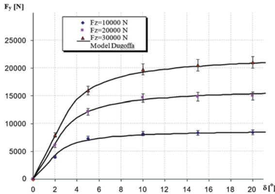
Fig. 4. Example of the tyres characteristics approximation determined when rolling a wheel with lateral drifting (tyre 255/70R22,5) [1]
