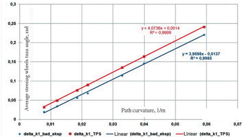
Fig. 6. Comparison of the  $L_c$  equivalent wheelbase for the 8x8 four-axle vehicle. Red line - course determined with the use of formula (7). Navy blue line - course determined on the basis of the experimental tests data
