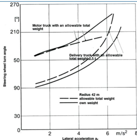
Fig. 1. Comparative characteristics of the truck vehicles steerability [3]
