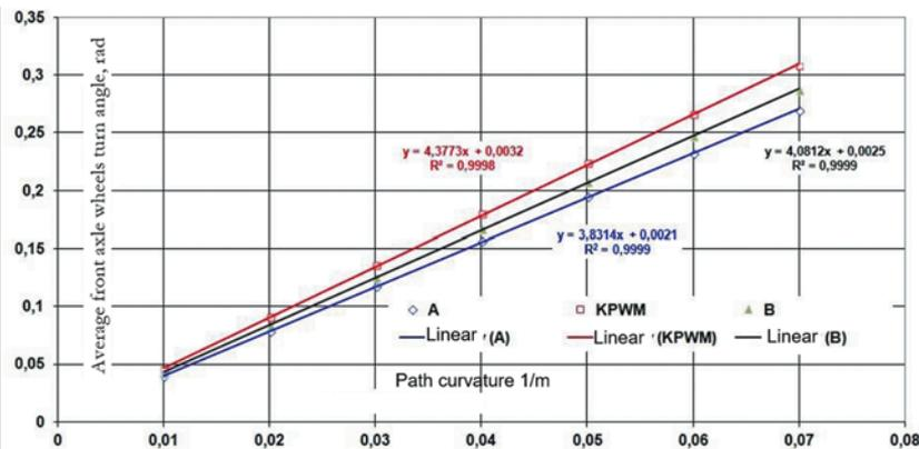
Fig. 5. Angular dependency of the  $\delta_1$ -front steering axle on the track curvature  $1/R$  for three-axle vehicles. The slop of the straight line constitutes the equivalent wheelbase  $y = L_e$  of the substitute two-axle vehicle (instead of  $L$  (2))
