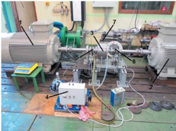
Fig. 1. Rig for the testing of driveline components. Object under test: a planetary gear unit.
