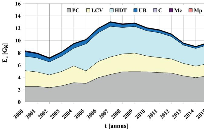
Fig. 14. Annual national emission of particulate matter PM<sub>2.5</sub> from tribological pairs of vehicles of specific cumulated categories
