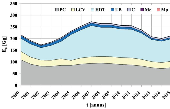
Fig. 13. Annual national emission of nitrogen oxides – NO<sub>x</sub> from vehicles of specific cumulated categories
