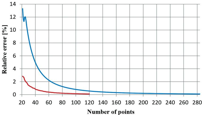
Fig. 11. Dependence of the relative length error after discretisation of the belt expressed as a function of the number of assumed points – a comparison of two assumed criteria:
