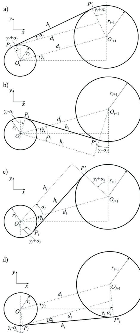
Fig. 3. Possible cases of two neighbouring pulleys with the belt
