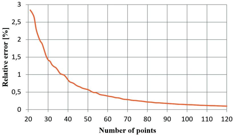
Fig. 8. Dependence of the relative length error after discretisation of the belt expressed as a function of the number of assumed points
