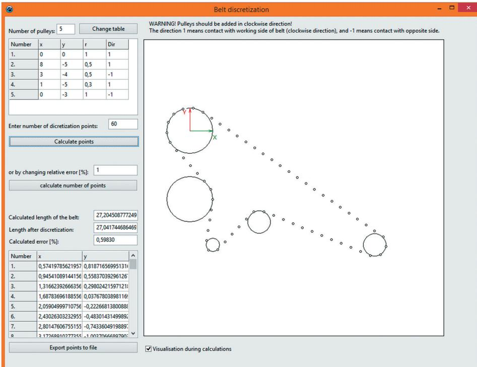
Fig. 6. Computer program developed for belt discretisation
