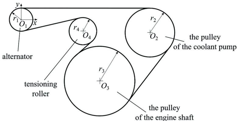
Fig. 7. Sample automobile transmission
