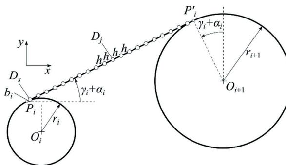
Fig. 4. Discretisation of the loose part of the belt between the wheels or rollers (case of contact of the working side of the belt on both wheels)
