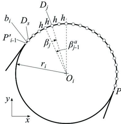
Fig. 5. Discretisation of the part of the belt that surrounds the pulley or roller (the case of the clockwise direction with the working side of the belt)
