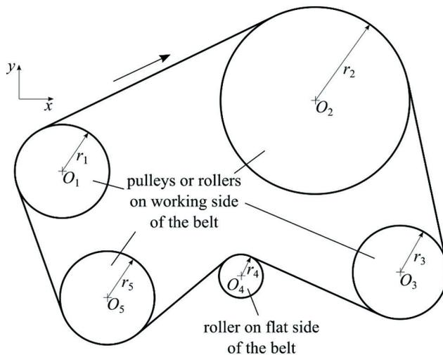
Fig. 2. The assumed order of pulleys and tensioning rollers shown based on an example of a four-pulley transmission with one tensioning roller
