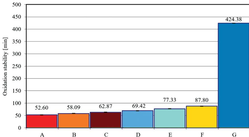
Fig. 1. Oxidation stability of the fuel samples under test
