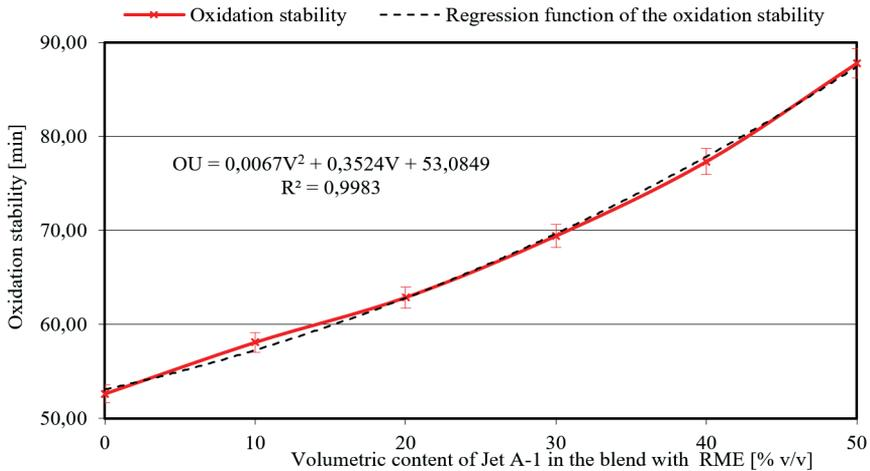
Fig. 3. Oxidation stability of the RME and Jet A 1 blends (with up to 50 % Jet A 1 content, by volume)
