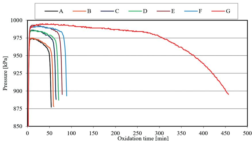
Fig. 2. Oxygen pressure in the reaction vessel with a sample of the fuel under test vs oxidation time
