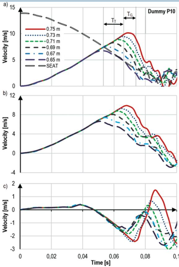
Fig. 7. Dummy P10 head velocity vs time curves for several seat spacing values:
