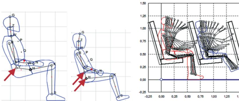
Fig. 4. Characteristic points on the models of the test dummies and their movements during the experiment; the arrows indicate the articulated joints that are important from the torso bending point of view
