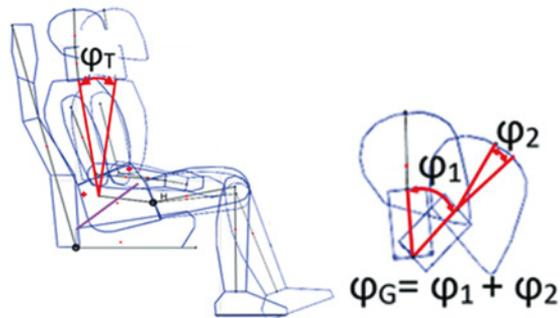
Fig. 6. Torso and head bend angles ( $\varphi_T$  and  $\varphi_G$ , respectively)
