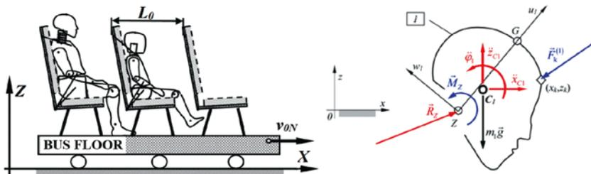
Fig. 2. General view of the model and the head loads (one of the options considered)
