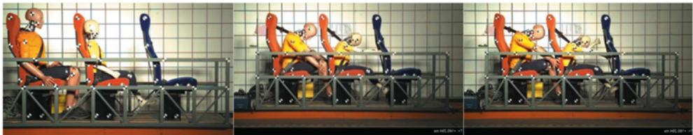
Fig. 3. Positions of dummies H III and P10 at successive instants (0-180 ms)
