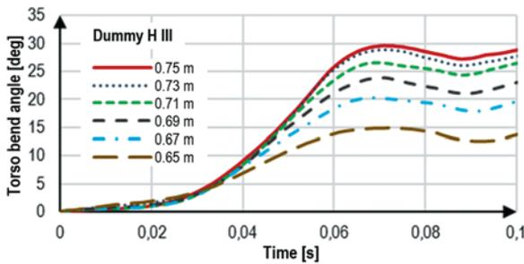
Fig. 12. Dummy H III torso bend angle  $\varphi_t$  vs time curves for several seat spacing values
