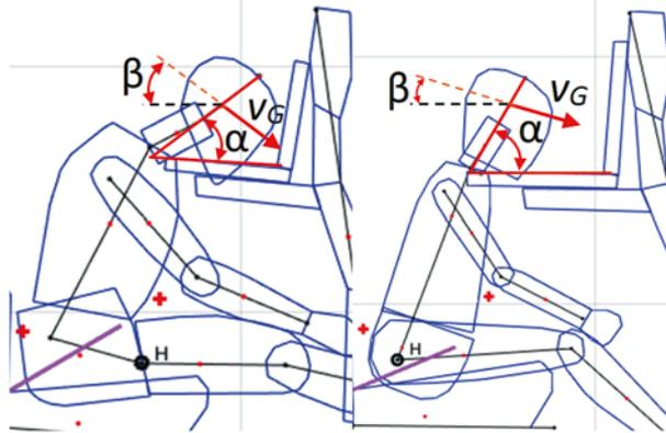
Fig. 13. Head bend angle relative to the mobile computer ( $\alpha$ ) and angle of inclination ( $\beta$ ) of the vector of resultant velocity  $v_G$  of the head mass centre of dummy H III (left) and P10 (right) at the instant of hitting on the computer
