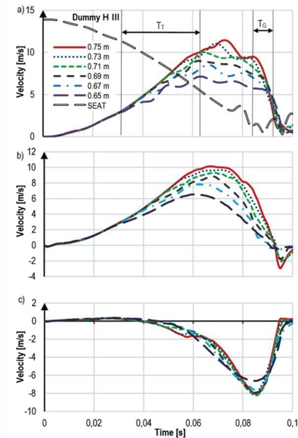
Fig. 10. Dummy H III head velocity vs time curves for several seat spacing values:
