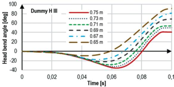
Fig. 11. Dummy H III head bend angle  $\varphi_c$  vs time curves for several seat spacing values
