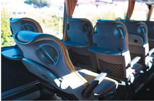
Fig. 1. Tables attached to bus seat backrests [13]
