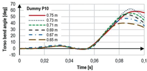
Fig. 9. Dummy P10 torso bend angle  $\varphi_T$  vs time curves for several seat spacing values
