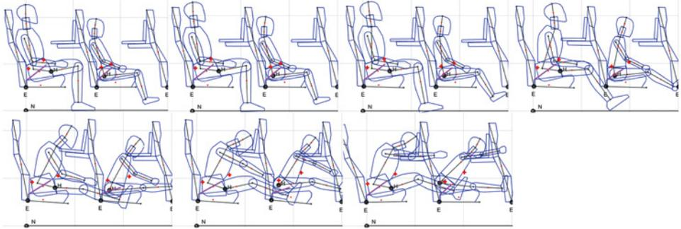
Fig. 5. Computer animation of the motion of bodies of a child and an adult for the time interval of 0-0.12 s (animation step 0.02 s);  $L_0 = 0.75$  m
