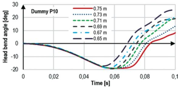
Fig. 8. Dummy P10 head bend angle  $\phi_G$  vs time curves for several seat spacing values
