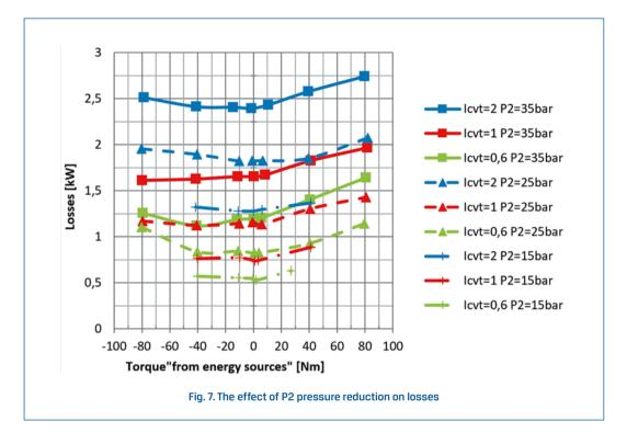
The obtained results clearly indicate that the smaller the P2 is, the smaller the losses are. However, this pressure cannot be reduced below the limit of permanent slip. For this reason, it is understandable to control the transmission in the area of micro-slip, which is described in more detail in [2].
