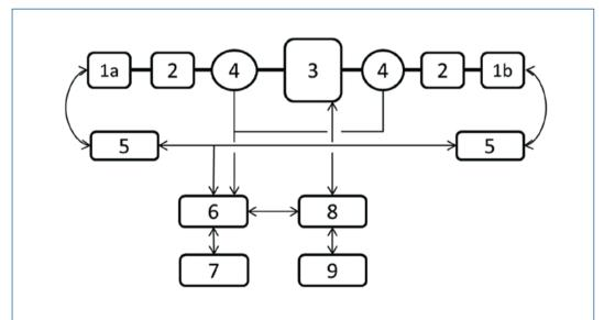
Fig. 4. Scheme of the test station; 1 – Electric machines; 2 – Mechanical transmissions; 3 – Tested continuously variable transmission; 4 – Torque metres; 5 – Inverters; 6 – Controller with an extensive input/output system; 7 – User interface; 8 – Hydraulic blocks (hydraulic distributors); 9 – Hydraulic group
