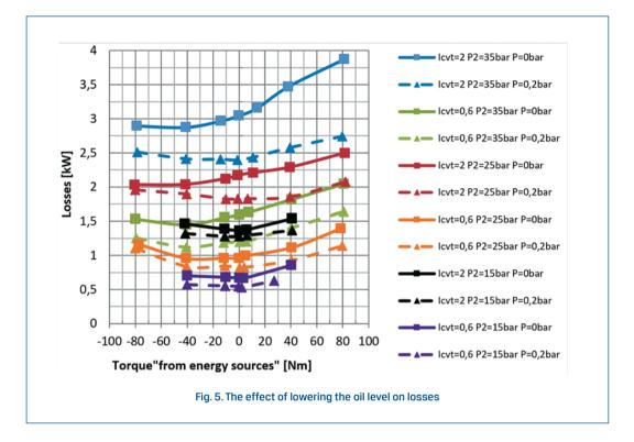
The relatively high value of the impact of wading losses indicates the need to look for structural solutions that allow to reduce these losses. In order to reduce these losses during the research, only cases with hypertension P = 0.2 bar will be presented in the further part of the article.
