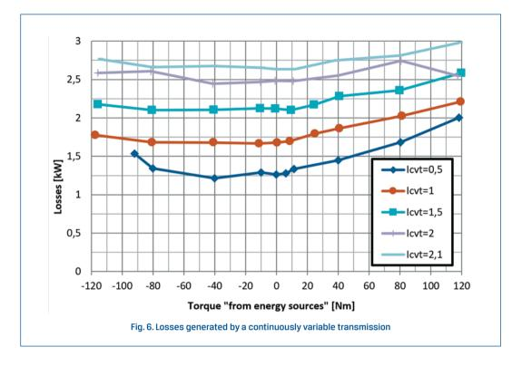
The losses generated are all the greater, the greater the transmission ratio and the larger the transmission (torque, both negative and positive). The decisive part of the losses is the part independent of the transmitted torque.
