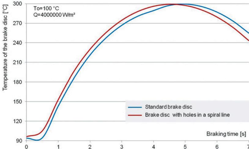
Fig. 4. Distribution of average temperature of brake discs after simulated braking.
