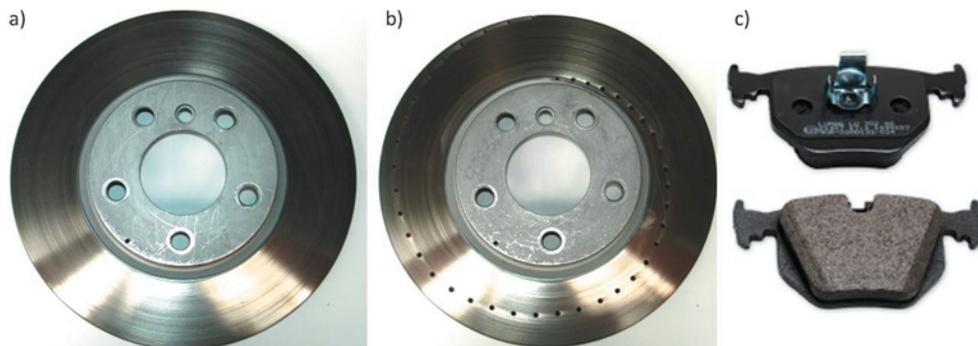
Fig. 6. View of the brake discs used during the test, a) standard disc (smooth), b) disc with holes in the spiral line, c) view of friction linings.
