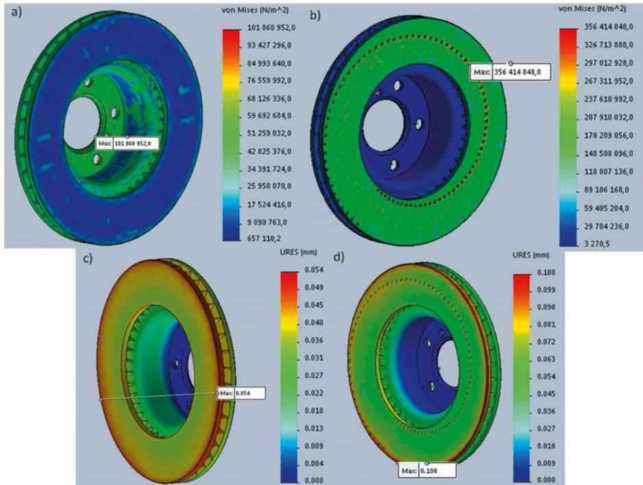
Fig. 5. Numerical analysis of von Mises reduced stresses for a standard disc without perforation, b) with holes in a spiral line and deformations c) for a standard disc, d) with holes in a spiral line
