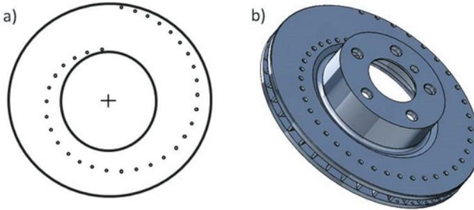
Fig. 2. Brake discs with holes in the Archimedes spiral line with one turn: a) diagram, b) disc model made in the SolidWorks 2016 environment.
