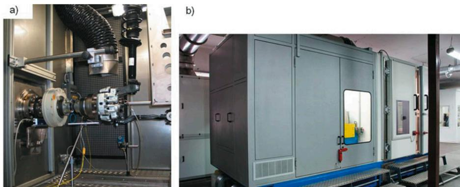
Fig. 7. View of the brake station at LUMAG, a) view of the test section with the calliper of the disc brake mounted, b) view of the driving part of the station with covered rotating masses of different inertia [10, 11].
