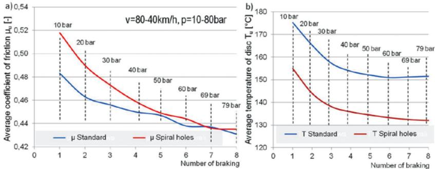
Fig. 9. The course of a) the average coefficient of friction, b) mean temperature of the disc as a function of successive braking ( $v = 80-40 \text{ km/h}$ ) for standard disc without perforation and disc with holes made in a spiral line for the *Speed/PressureSensitivity* test.
