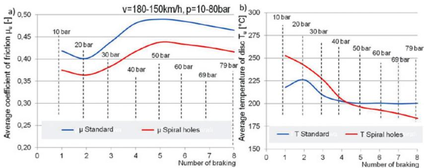
Fig. 12. The course of a) the average coefficient of friction, b) the mean temperature of the disc as a function of successive braking ( $v = 180-150\text{km/h}$ ) for the standard disc without perforation and the disc with holes made in a spiral line for the *Speed/PressureSensitivity* test.
