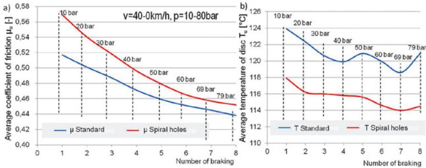
Fig. 8. The course of a) the average coefficient of friction, b) the mean temperature of the disc as a function of subsequent braking ( $v = 40-0 \text{ km/h}$ ) for the standard disc without perforation and the disc with holes made in a spiral line for the *Speed/PressureSensitivity* test.
