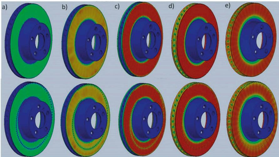
Fig. 3. Distribution of temperature on smooth disc (without perforation of friction surface) and disc with holes made in a spiral line after simulated braking lasting 7 seconds at the moment of time: a) 1s, b) 2s, c) 3s, d) 6s, e) 7s.
