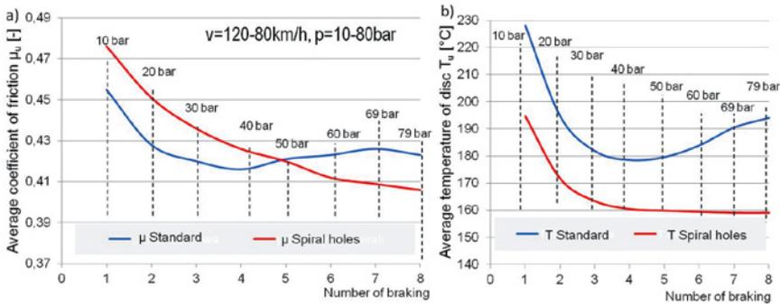
Fig. 10. The course of a) the average coefficient of friction, b) the mean temperature of the disc as a function of successive braking ( $v = 120-80\text{km/h}$ ) for the standard disc without perforation and the disc with holes made in a spiral line for the *Speed/PressureSensitivity* test.
