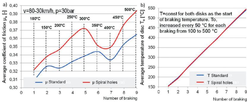
Fig. 14. The course of a) the average coefficient of friction, b) mean temperature of the disc as a function of successive braking ( $v = 180-150\text{km/h}$ ) for standard disc without perforation and disc with holes made in a spiral line for the *Increasing Temperature* test 500°C.
