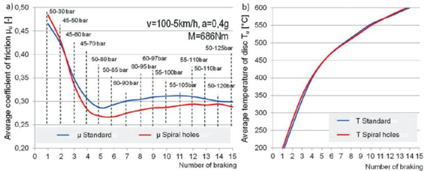
13. The course of a) the average coefficient of friction, b) mean temperature of the disc as a function of successive braking ( $v = 180-150\text{km/h}$ ) for the standard disc without perforation and the disc with holes made in a spiral line for the *Fading* test.
