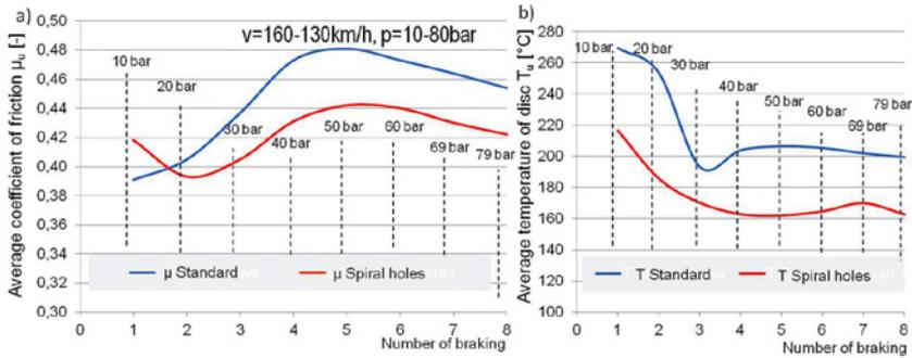
Fig. 11. The course of a) the average coefficient of friction, b) mean temperature of the disc as a function of successive braking ( $v = 160-130\text{km/h}$ ) for standard disc without perforation and disc with holes made in a spiral line for the *Speed/PressureSensitivity* test.
