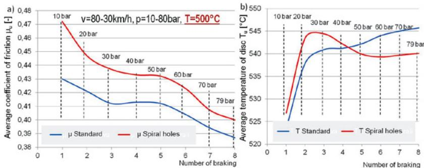
Fig. 15. The course of a) the average coefficient of friction, b) the mean temperature of the disc as a function of successive braking ( $v = 180\text{-}150\text{km/h}$ ) for the standard disc without perforation and the disc with holes made in a spiral line for the *Pressure Line* 500°C test.
