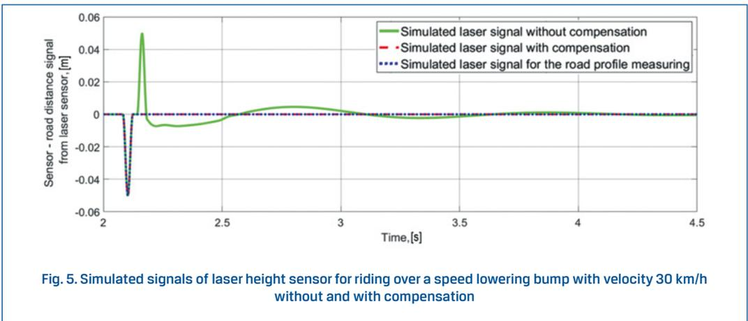
Fig. 5. Simulated signals of laser height sensor for riding over a speed lowering bump with velocity 30 km/h without and with compensation
