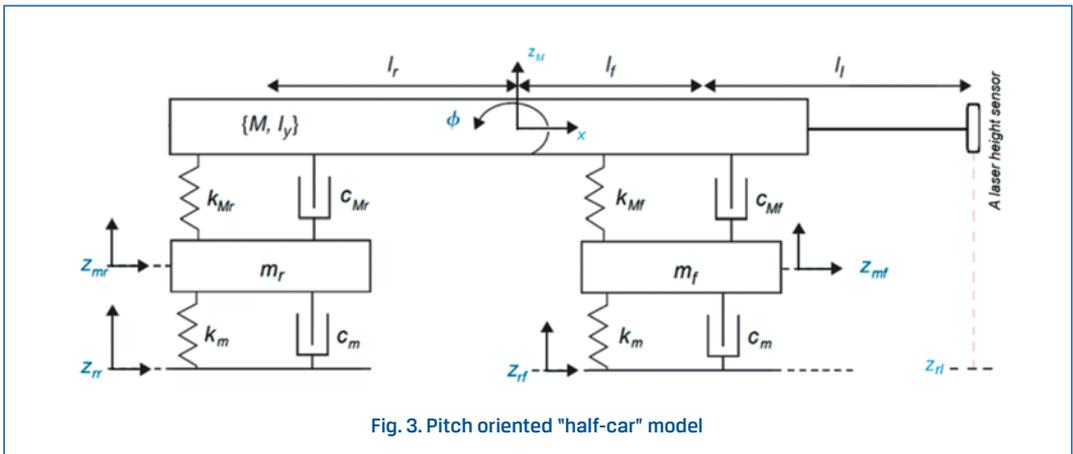
The "half-car" model (Fig. 3) consists of three bodies:  $M$  – vehicle's body (sprung mass),  $m_f$  or  $m_r$  – the front and rear wheels with axles (unsprung masses). This model has 4 degrees of freedom: the vertical displacement of sprung mass  $z_M$  and transverse about the transverse axis  $\phi$ , the displacements of the unsprung masses  $z_{mr}$  and  $z_{mf}$ .
