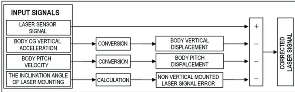
Fig. 2. Laser height sensor signal compensation for vehicle body dynamics
