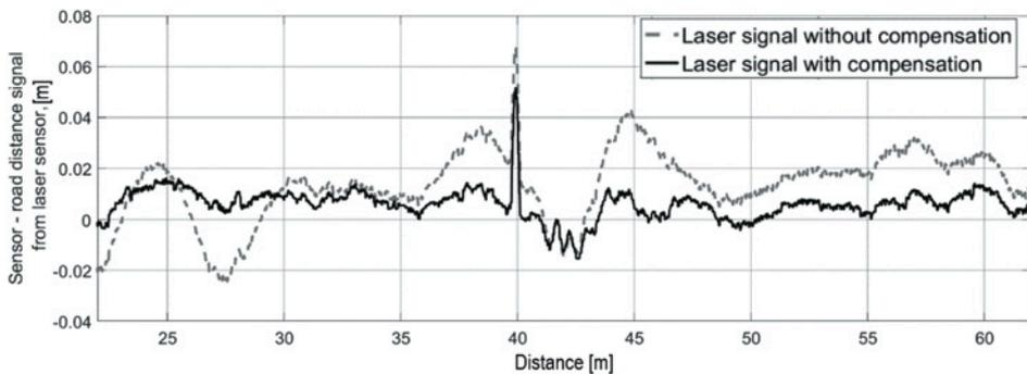
Fig. 8. The road profile estimation using laser sensor No. 1 – comparison of a raw sensor signal and compensated with proposed algorithm – soft damping case
