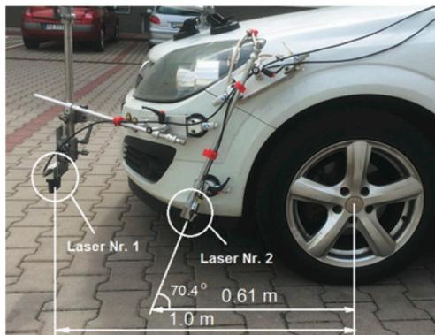
Fig. 6. Laser sensor mounting positions
