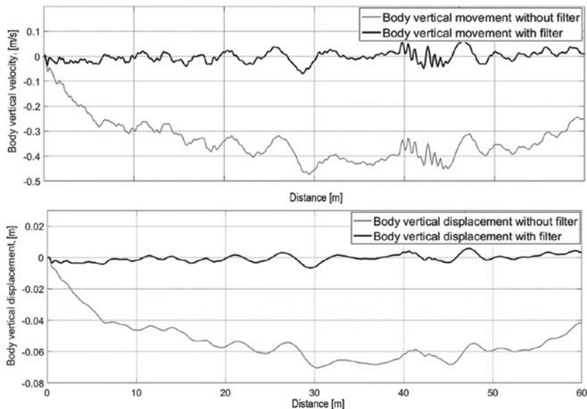
Fig. 7. Estimation of the vehicle body displacements
