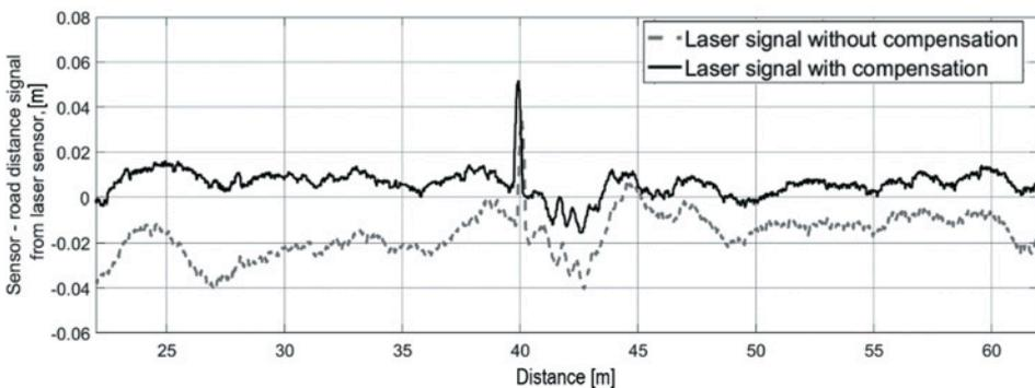
Fig. 9. The road profile estimation using laser sensor No. 1 – comparison of a raw sensor signal and compensated with proposed algorithm – stiff damping case
