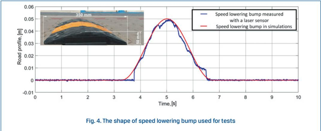
Fig. 4. The shape of speed lowering bump used for tests
