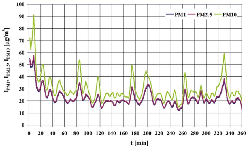
Fig. 5. The immission of particulate matter PM1, PM2.5, and PM10 (data recorded by the Dust Trak DRX Aerosol Monitor and smoothed by filtration) [14]
