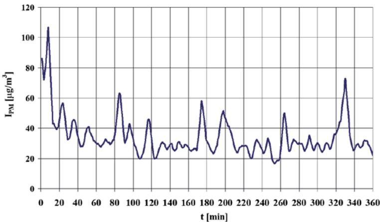
Fig. 3. The TSP immission (data recorded by the Dust Trak DRX Aerosol Monitor and smoothed by filtration) [14]
