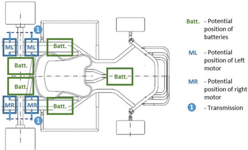
Fig. 6. Potential position of the main components of eKart
