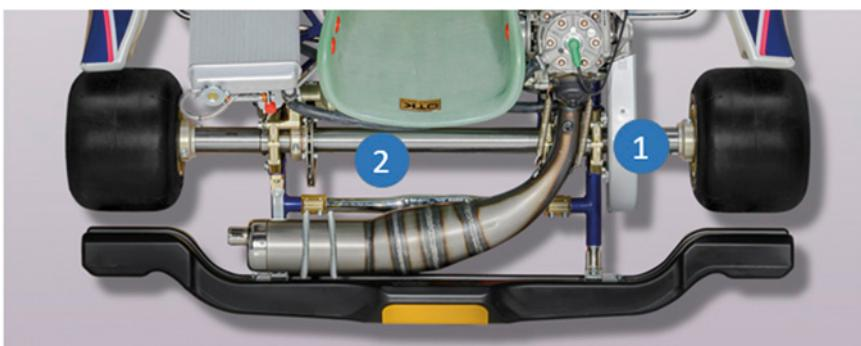
Fig. 5. Rear Suspension elements of Kosmic MERCURY MY15 [11]
