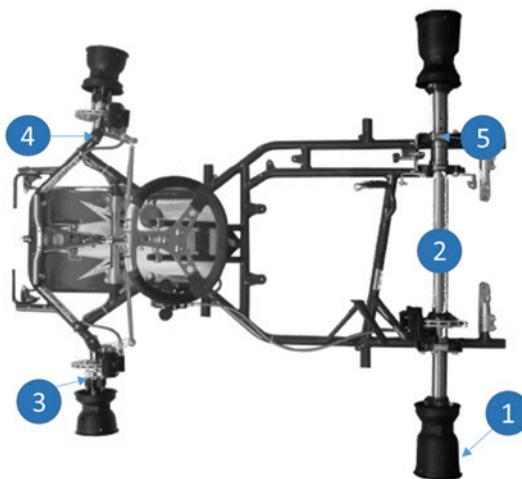
Fig. 1. ICE Gokart chassis Birel type RY 30 and its main component [7] [8]
