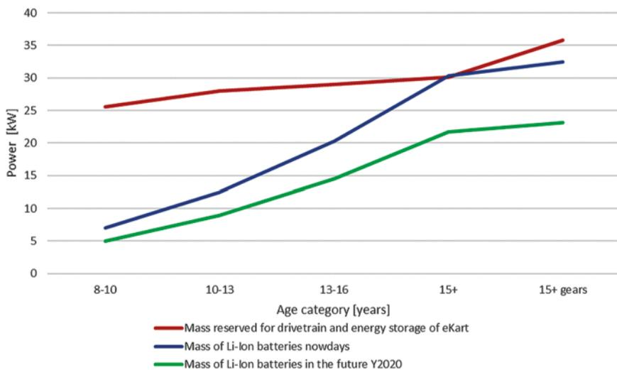
**Fig 3 Maximum weight of drivetrain unit of eKart with batteries compared to potential mass of the batteries in Li-Ion technology nowadays and in 3 years' time for given age categories**
