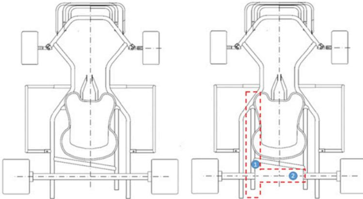
Fig. 4. Sketch of modification of the ICE gokart chassis for the eKarta construction
