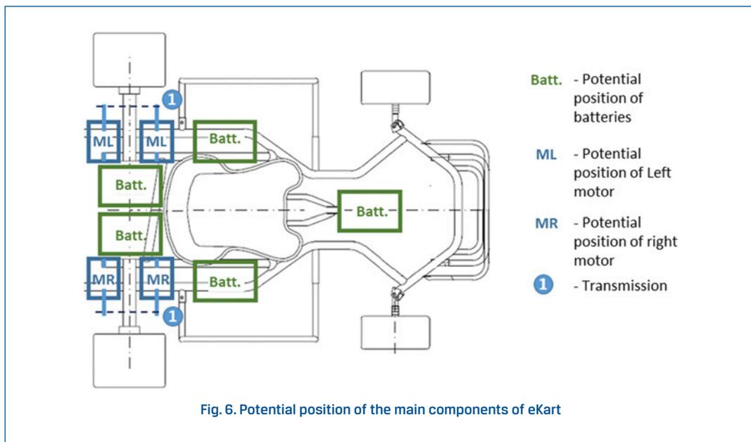
eKart will be equipped with Electric motors of different power depending on the age category. There can be also different kind of motor cooling, air cooled and liquid cooled, depending on its power.
