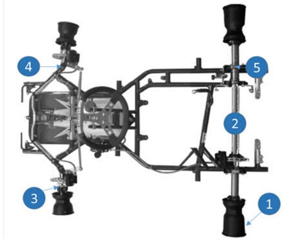
Fig. 1. ICE Gokart chassis Birel type RY 30 and its main component [7] [8]
