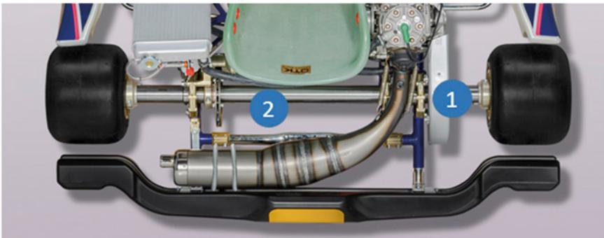
Fig. 5. Rear Suspension elements of Kosmic MERCURY MY15 [11]
