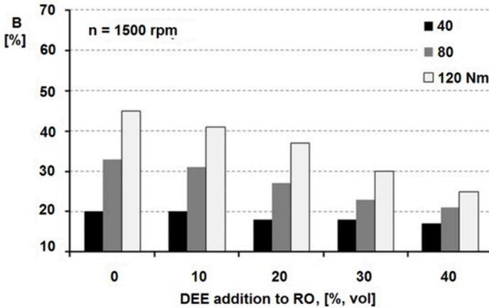
Fig. 3. Impact of DEE addition to RO on smoke emission of AD3.152 engine operated at 1500 rpm
