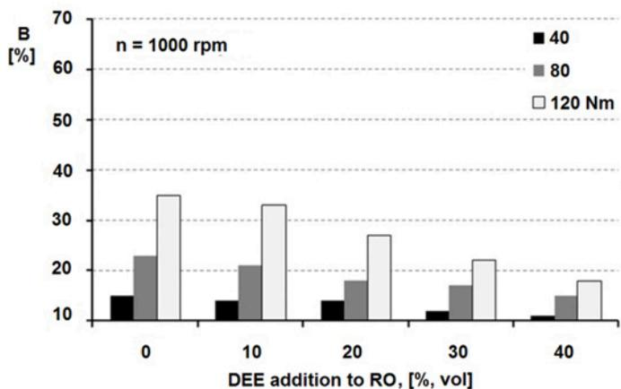
Fig. 2. Impact of DEE addition to RO on smoke emission of AD3.152 engine operated at 1000 rpm
