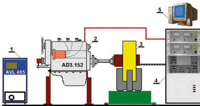
Fig. 1. Test stand scheme: 1 – AVL465 gas analyzer, 2 – AD3.152 engine, 3 – engine brake, 4 – steering box, 5 – PC workstation
