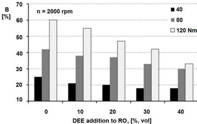
Fig. 4. Impact of DEE addition to RO on smoke emission of AD3.152 engine operated at 2000 rpm.
