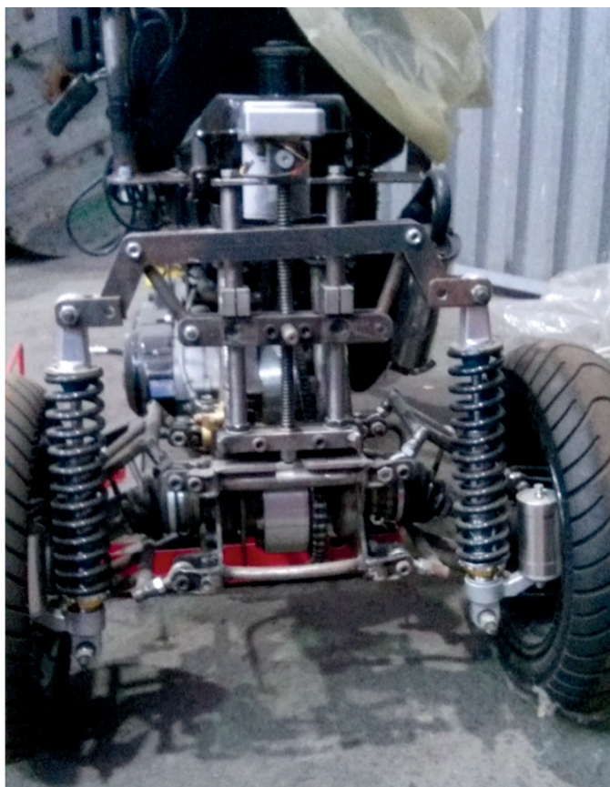
Fig. 1. Three-wheeler with the independent rear wheels suspension system
