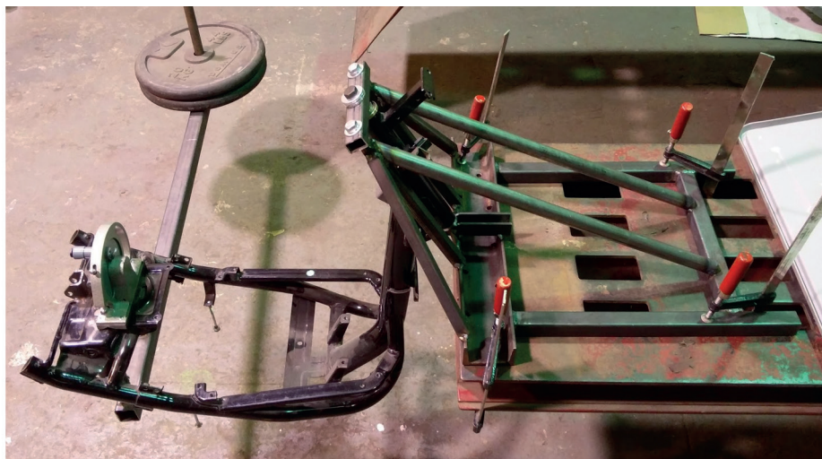
Fig. 14. Test rig for determining the torsional stiffness of the frame of a three-wheeled vehicle
