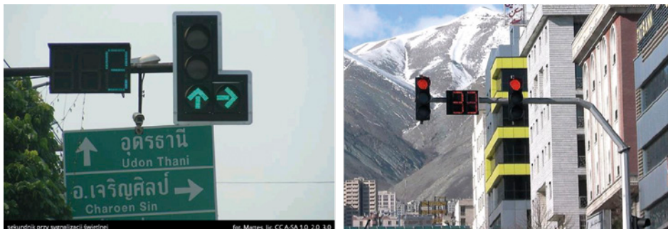
Fig. 3. Traffic lights with countdown timers in Thailand [13] and in Iran (Tehran) [12]
