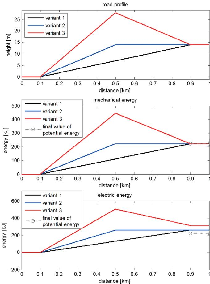
**Fig. 7. Comparison of mechanical energy requirement and electrical energy supplied to motor to overcome grade resistance for road profiles of same average grade**
