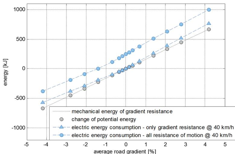
Fig. 8. Electric energy consumption from different road grade on test section
