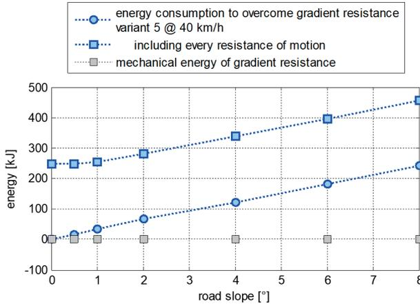
Fig. 9. Impact of road inclination on test section with average inclination equal zero on electric energy consumption
