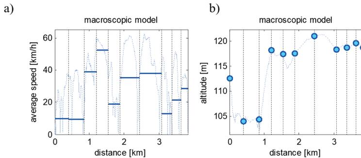
Fig. 4. Input data for macroscopic model - average speed per section and road altitude at nodes
