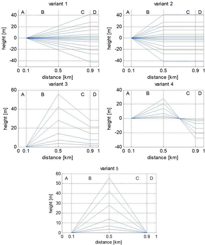
Fig. 5. Road profiles used in simulation study variants 1-5.
