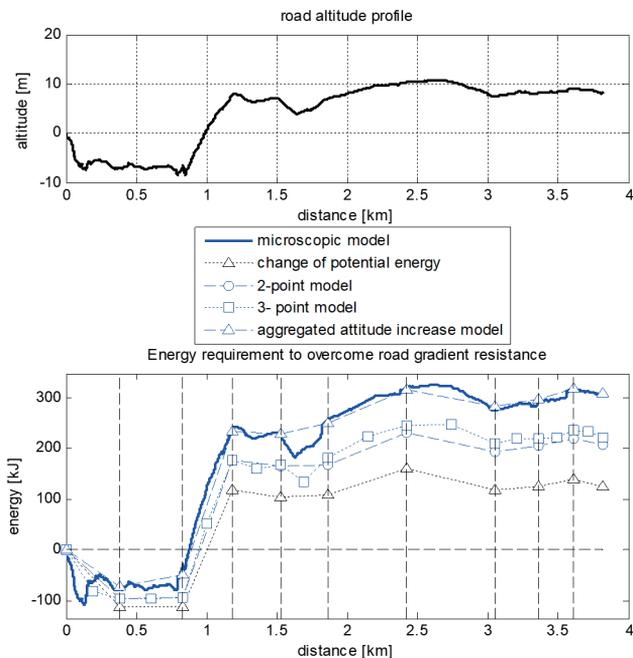
Fig. 11. Comparison of estimation of energy required to overcome grade resistance obtained from different models
