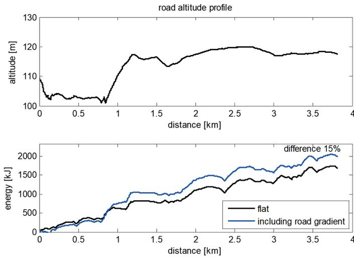
Fig. 3. Example of road profile and difference between energy consumption between estimation with and without grade resistance
