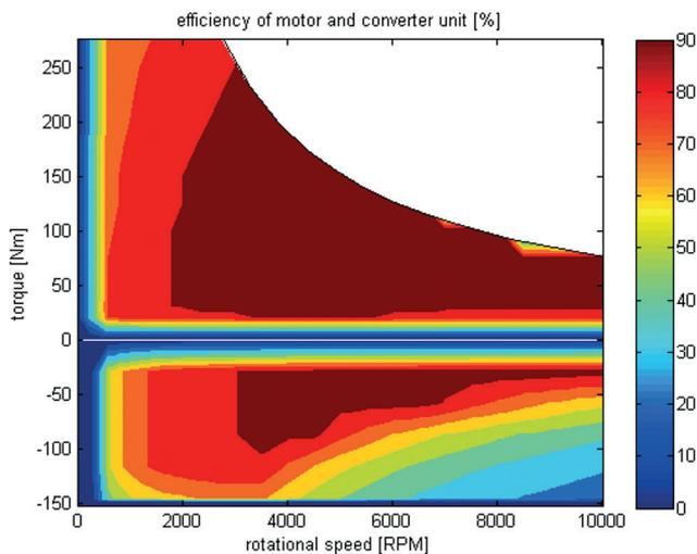
Fig. 6. Efficiency of motor and converter used in microscopic model
