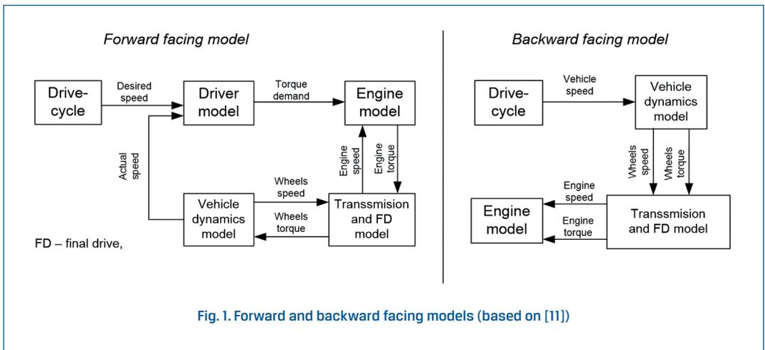
Fig. 1. Forward and backward facing models (based on [11])
