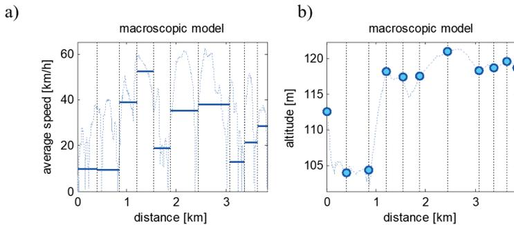
Fig. 4. Input data for macroscopic model – average speed per section and road altitude at nodes
