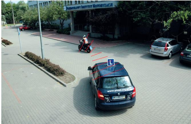
Fig. 10. Radio system for training and examining a deaf motorcyclist with using vibrating command points installed on a special harness worn by him/her [5]
