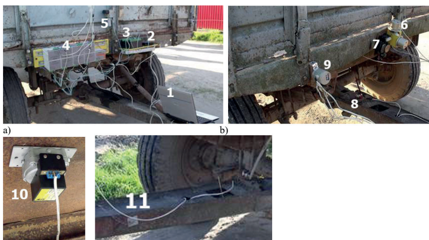
Fig. 7. Three-unit vehicle with the measuring equipment 's complex. (a-d) 1) Integrated into the measuring complex of the stand alone PC with software based on a laptop. 2) Modem for data transmissions 3) module analog digital transformer – digital analog transformer with galvanic decoupling lines of digital input and output 4) power supply units for sensors 5, 7) sensors of linear displacement between truck and first trailer and first trailer and second trailer 6) vibration sensors 8) sensor of angular displacement 9) speed sensors 10) accelerometer, 11) tenzo sensor
