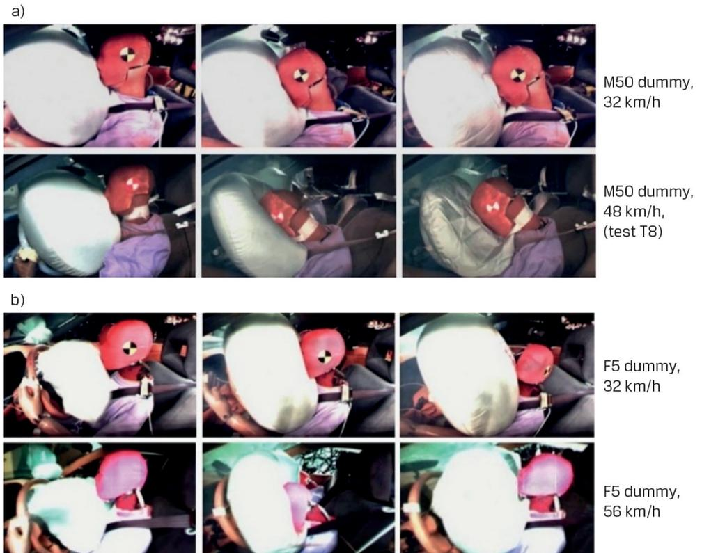
**Fig. 9.** The displacements of the dummy in respect of the airbag in the same car model (elaborated on the basis of [24]); a) M50 dummy, 32 and 48 km/h; b) F5 dummy, 32 and 56 km/h
