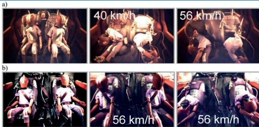
**Fig. 10.** The displacements of the 6YO dummies in the back seats (elaborated on the basis of [24]);
