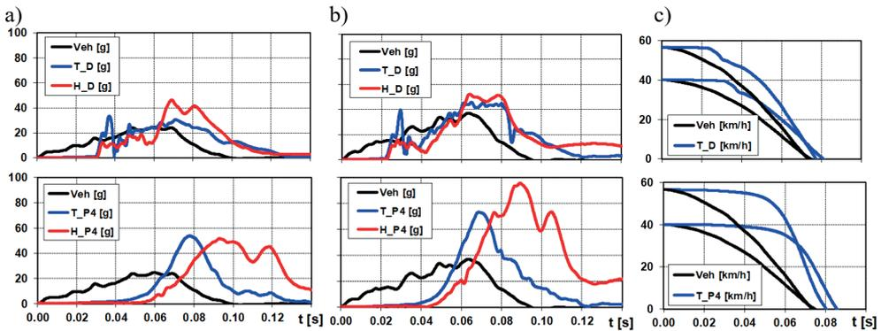
Fig. 4. The performances of the deceleration that acts on the car (Veh), torso (T) and head (H) of the F5 dummy in the driver's seat (D) and in the back seat (P4) in the T6 tests; a) velocity 40 km/h, b) velocity 56 km/h, c) performances of the car velocity and dummy torso
