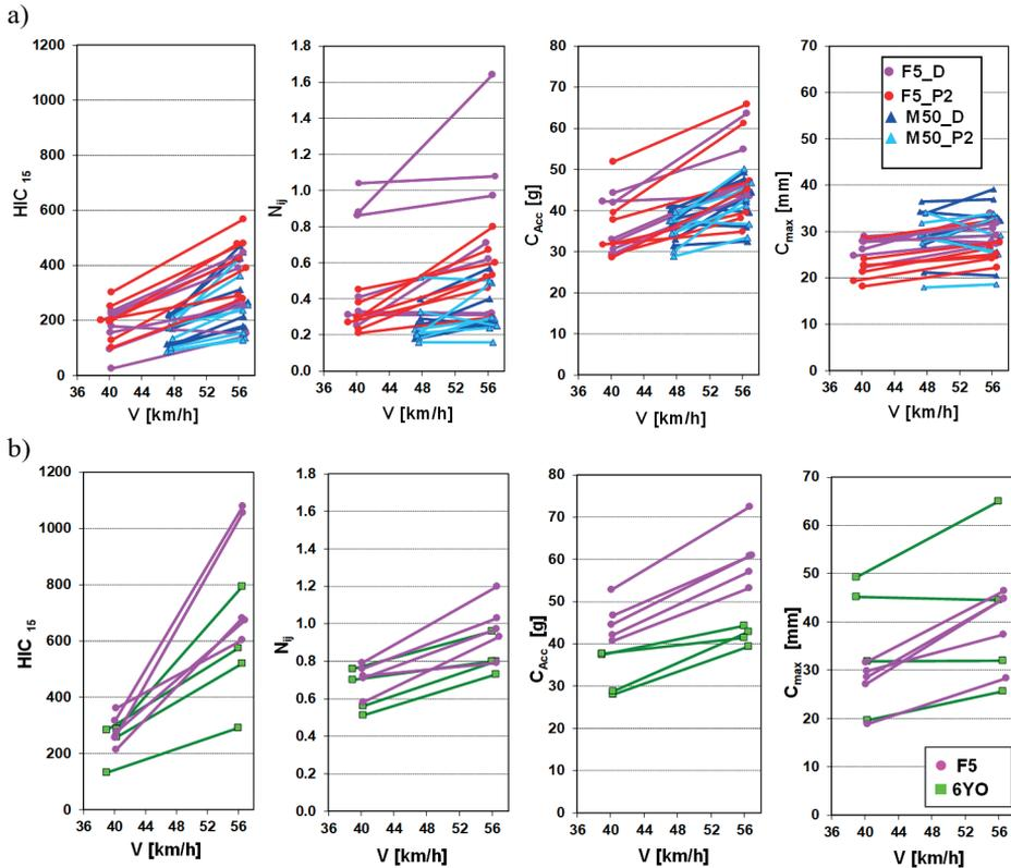
**Fig. 5. The values of the injury criteria in the function of the impact velocity;**
