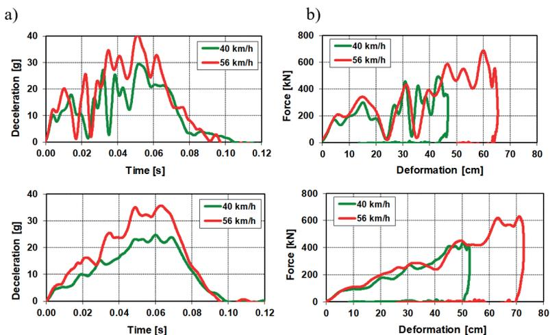
Fig. 3. The performances of the car decelerations and deformation characteristics (T1 and T6 tests)
