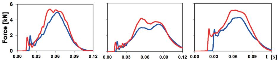
Fig. 8. The performances of the tensile force of the driver's seat belt webbing (the F5 dummy) in the T1, T2 and T6 tests
