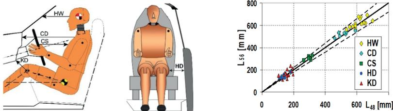
Fig. 2. The dimensions describing a position of the dummy in the car – the dotted lines on the graph determine an interval of  $\pm 10\%$  (on the basis of [24])
