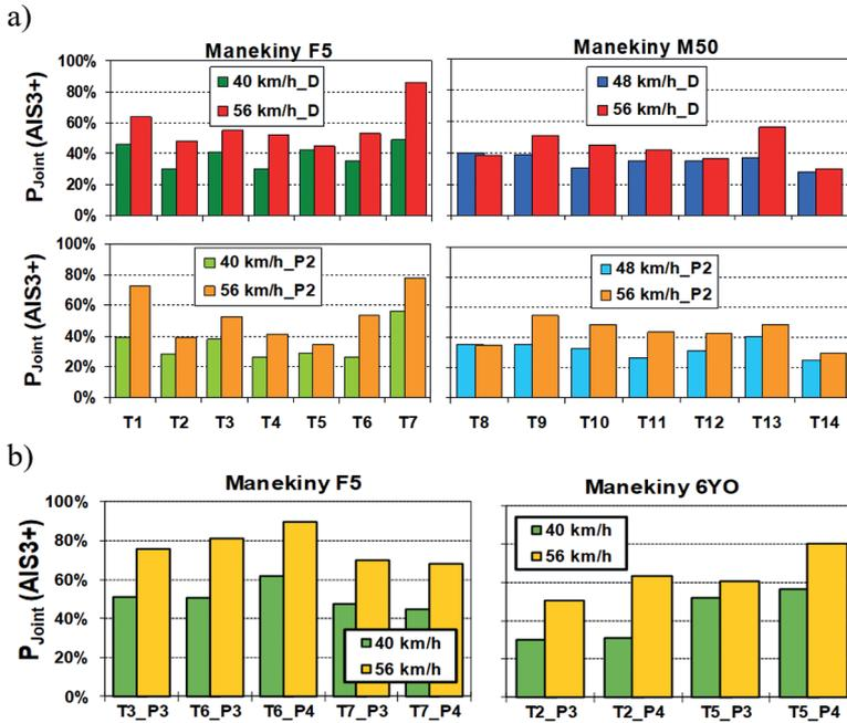
Fig. 7. Influence of the impact velocity on the AIS3+ risk injury; a) of the driver (D) and the passenger (P2), b) passengers in the back seats (P3 and P4)
