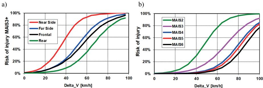
Fig. 1. The influence of the change in car velocity during the collision on the injury risk [2, 16]
